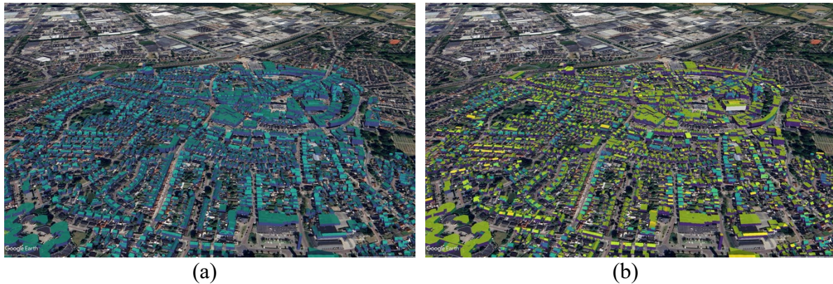
Figure 4. Rijssen-Holten solar irradiance output visualisation in May for NTA880 (a) and our computation (b).
