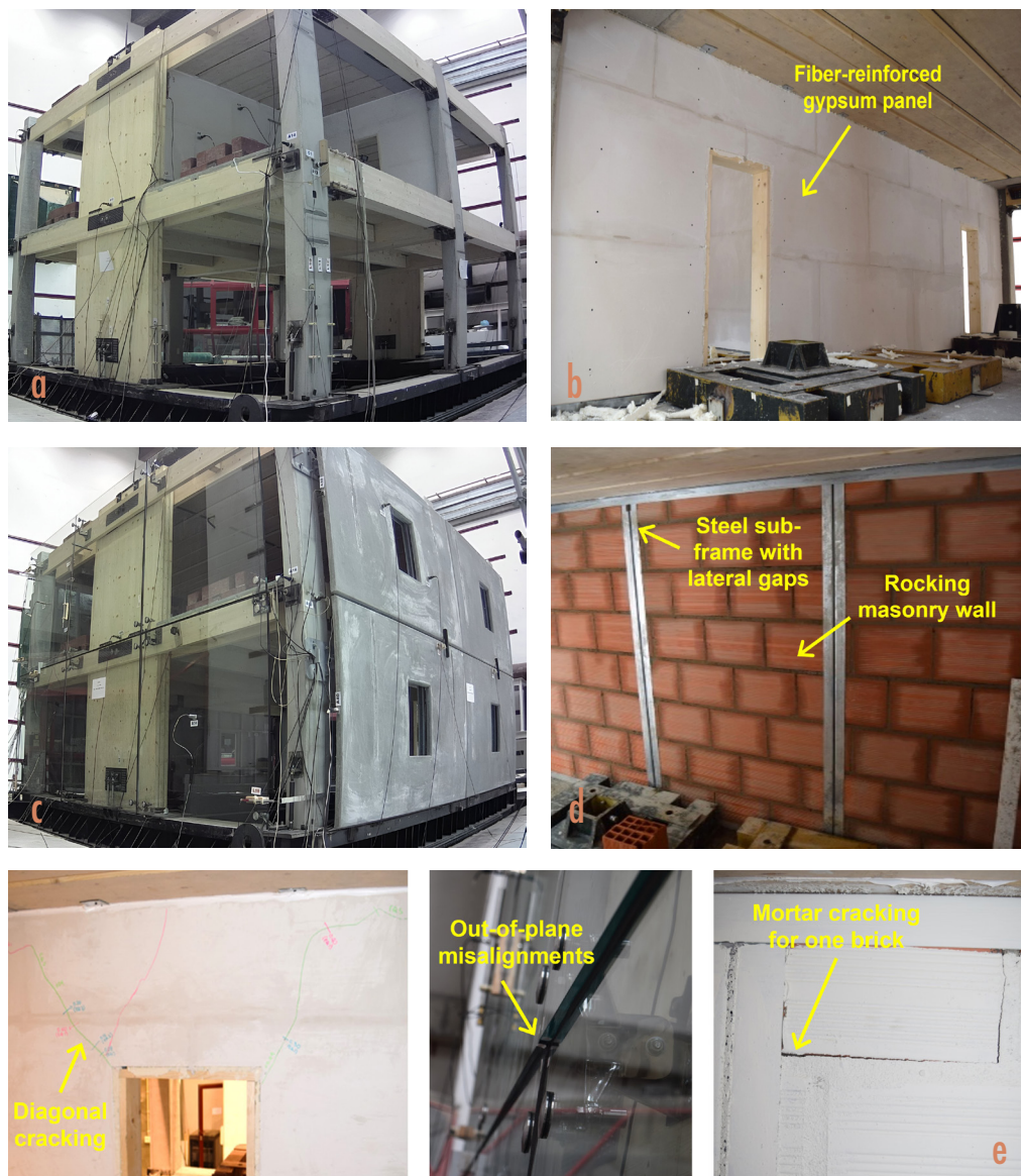
Figure 4. (a, b) Specimen configuration including a low-damage drywall partition on the first floor; (c, d) Integrated building configuration with concrete and glazed façades, and an internal low-damage masonry wall. (e) Observed non-structural damage.
