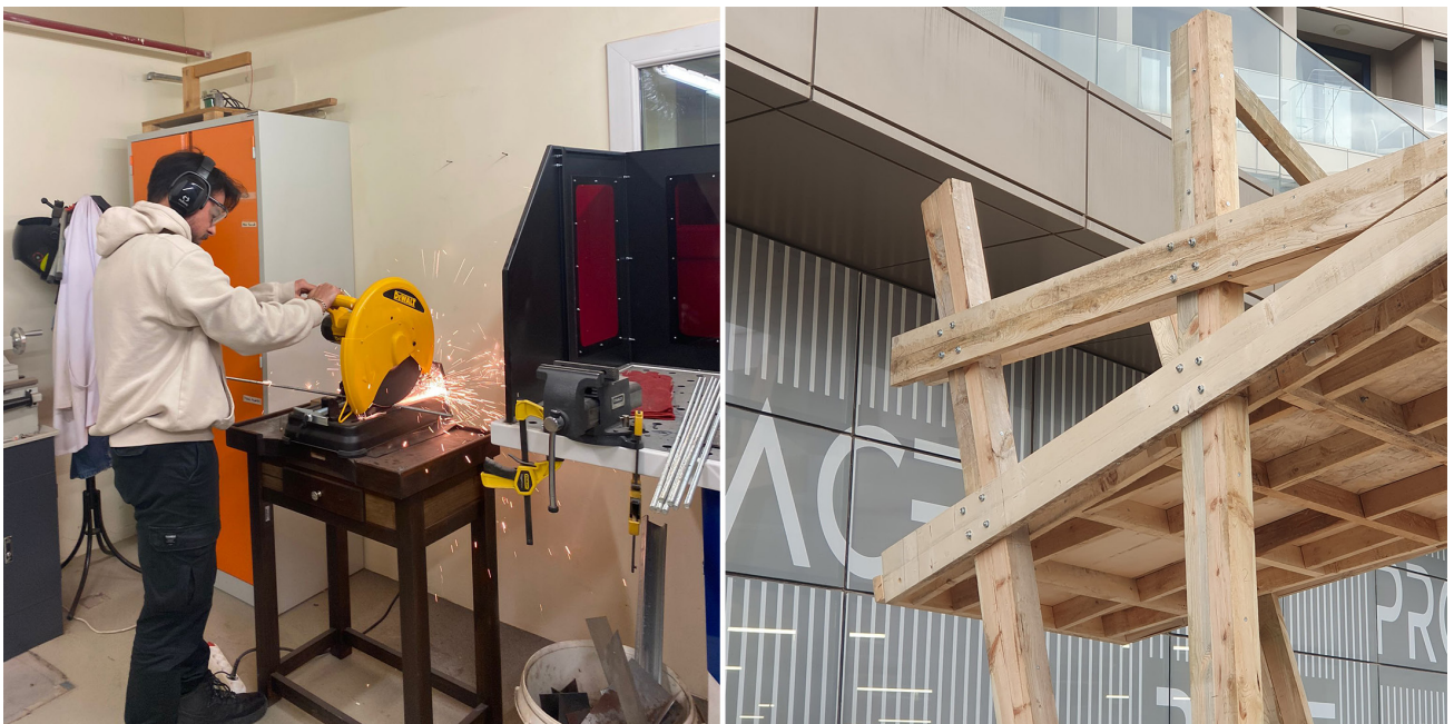
Figure 10. Cutting the metal rods for producing bolt connections to be used in the assembly process.
