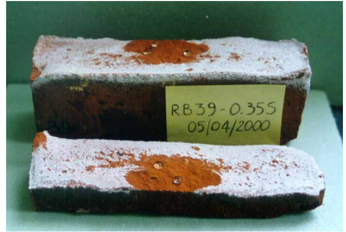
FIGS. 4.12/4.13 Salt accumulation beneath the layer treated with a water repellent (left) and subsequent spalling of the treated part (right) during a laboratory test / Photos: B. Lubelli
