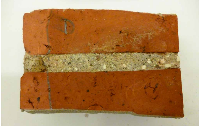
FIG. 4.26 The penetration depth of a water repellent treatment has been assessed by wetting a cross section of the sample with water: the light part corresponds with the treated layer / Photo: B. Lubelli
