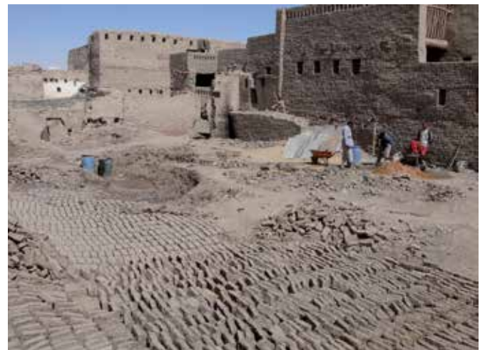
FIG. 2.1 Fabrication of brick, Qasr in Daklah (Egypt) / photo: D. Schultz
