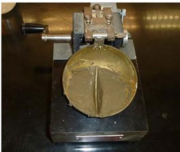
*Casagrande cup with sample in which a groove has been made.*
