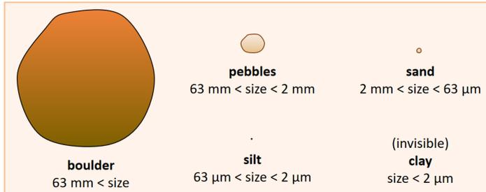
Traditionally, sieves could not be made for particle sizes smaller than 63 μm. This is why the lower limit of 63 μm was adopted for sand. The size of silt particles is measured traditionally by **hydrometer** test. Nowadays, **Static Light Scattering** (laser diffraction) devices enable to measure the whole range of particle sizes (from 1 nm to 1 mm) with a single device, see **Chapter 2**.
