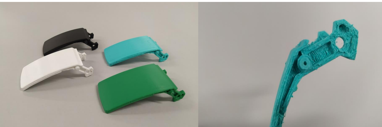
Figure 29 - Same part printed in different materials, resulting in differences in surface quality. (right) Surface quality with PETG filament without following the TDS printing recommendations.
