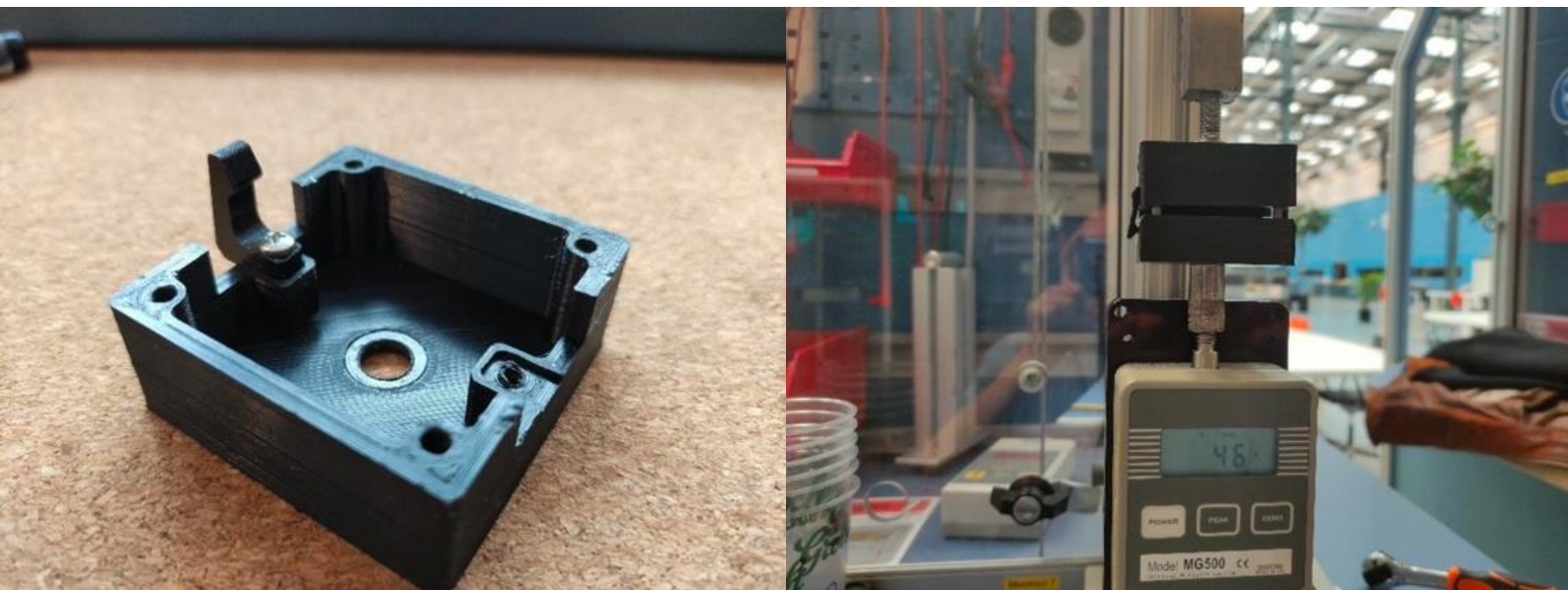
Figure 31 - (left) Jig and (right) force gauge with jig installed to measure tensile and compression forces on snap fits. Used with approval of M. Bakker, 2021.
