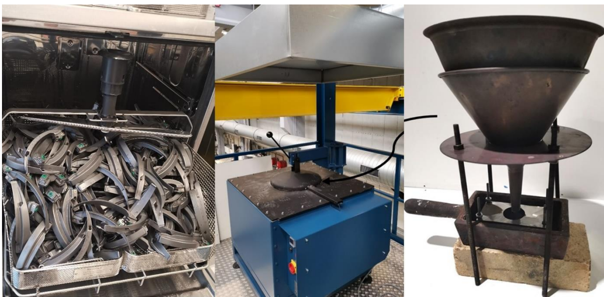
Figure 2. Cleaning, disinfection, melting and casting Zamak. Left: the cleaning and disinfection machine. Middle: the melting oven. Right: the casting set-up. Photo by Bart van Straten.
