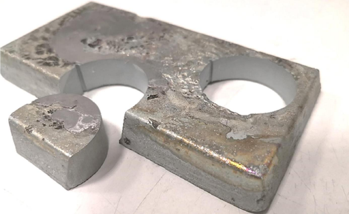
Figure 3. Zamak bar, cast from recycled laryngoscope blades. Round parts were cut from the bar and processed into usable material. Photo by Bart van Straten.
