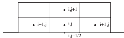
Figure 4.6: Control volume for the cell-centered Robin boundary condition.
