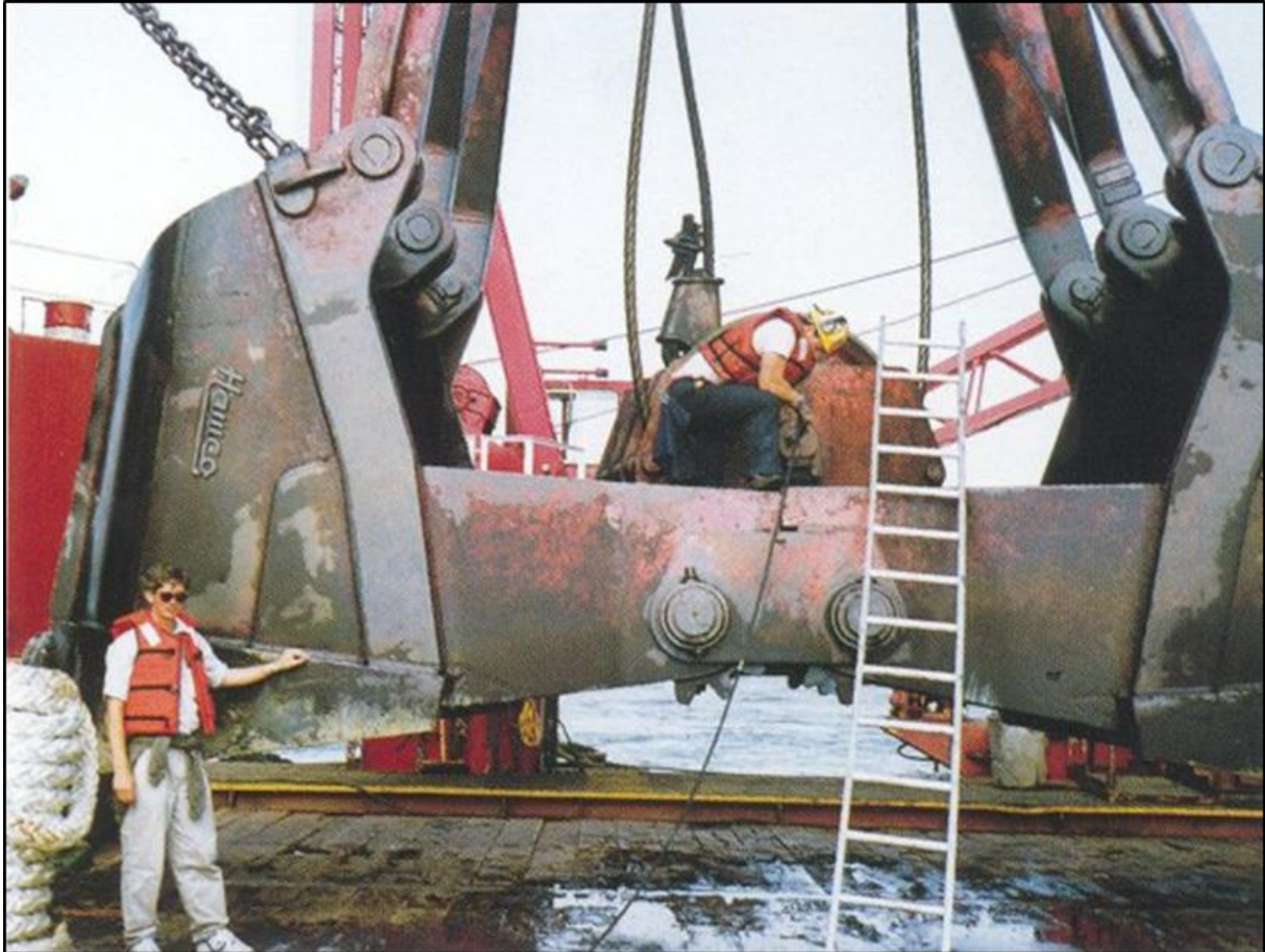
Figure 1-3: The author on the clamshell dredge “Chicago” of Great Lakes Dredge & Dock.
