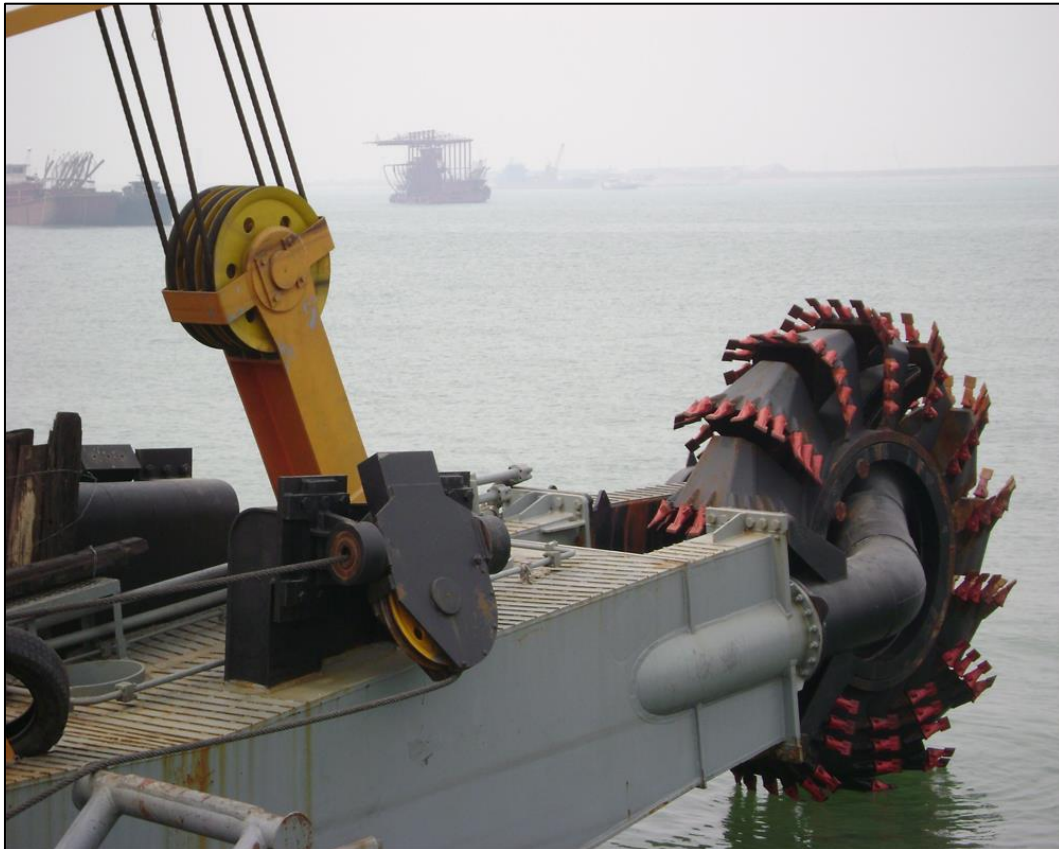
Figure Y-38: A bucket wheel dredge (China Hi Sea).
