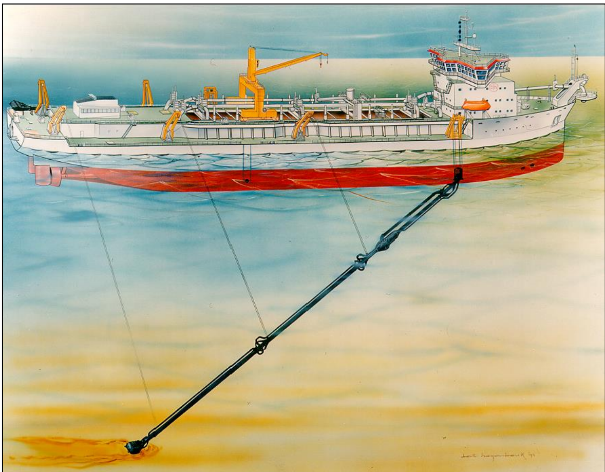
Figure Y-18: The Gerardus Mercator (Jan de Nul, 18000 m 3 ) with one drag arm.
