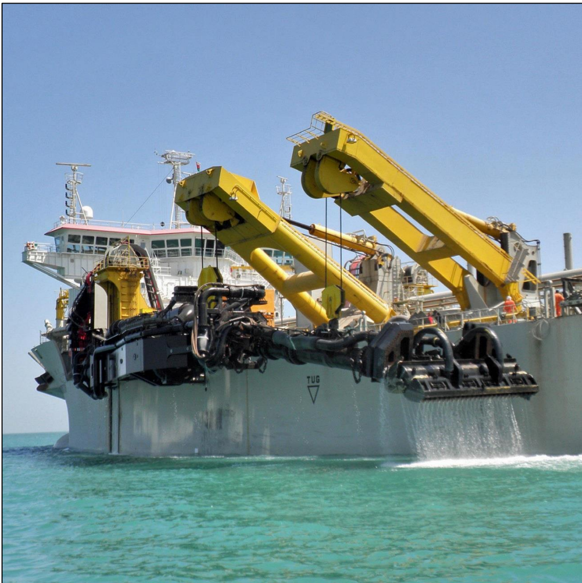
Figure Y-22: TSHD suction pipe (Jan de Nul).
