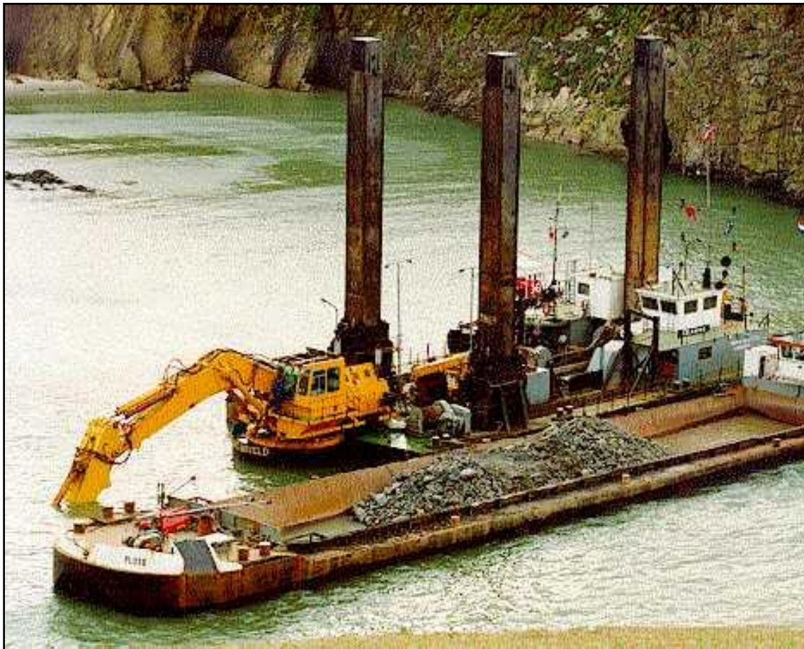
Figure Y-27: A large backhoe dredge.
