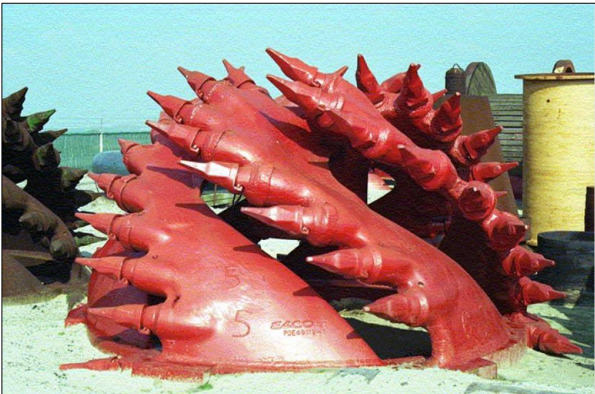
Figure Y-16: Rock cutterhead (IHC).
