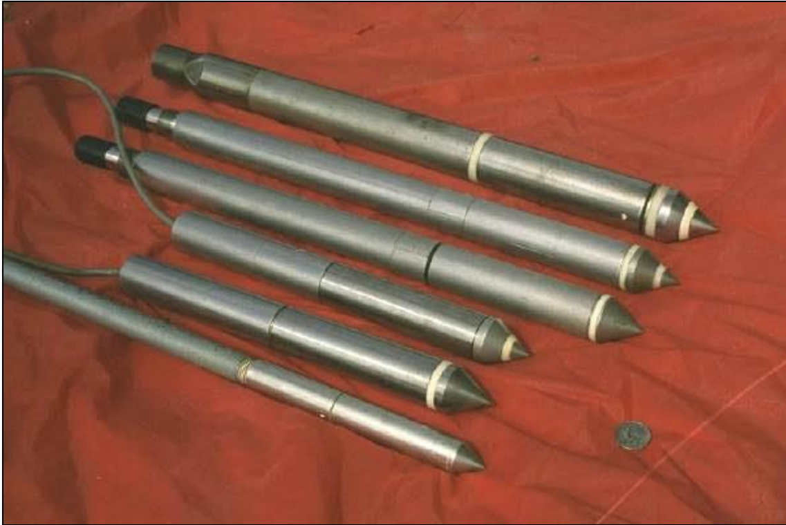
Figure 2-34: Several cone configurations.
