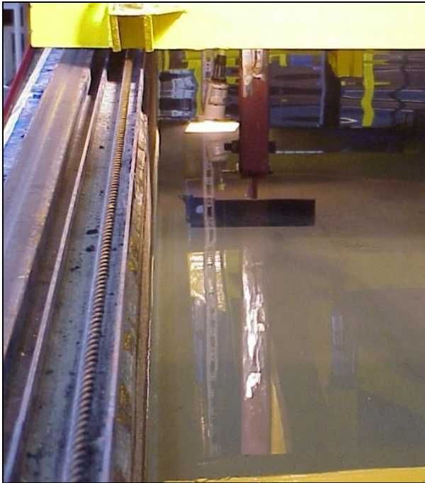
Figure 12-31: The blade mounted under the carriage
