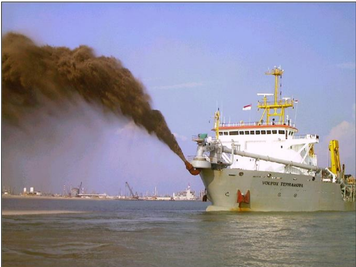
Figure Y-20: The Volvox Terranova rainbowing (van Oord).
