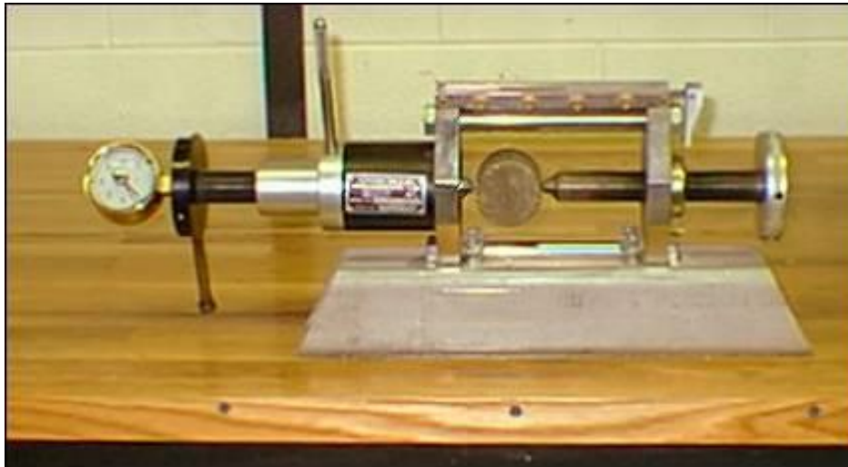
Figure 2-40: Point load test facility (inside.mines.edu).
