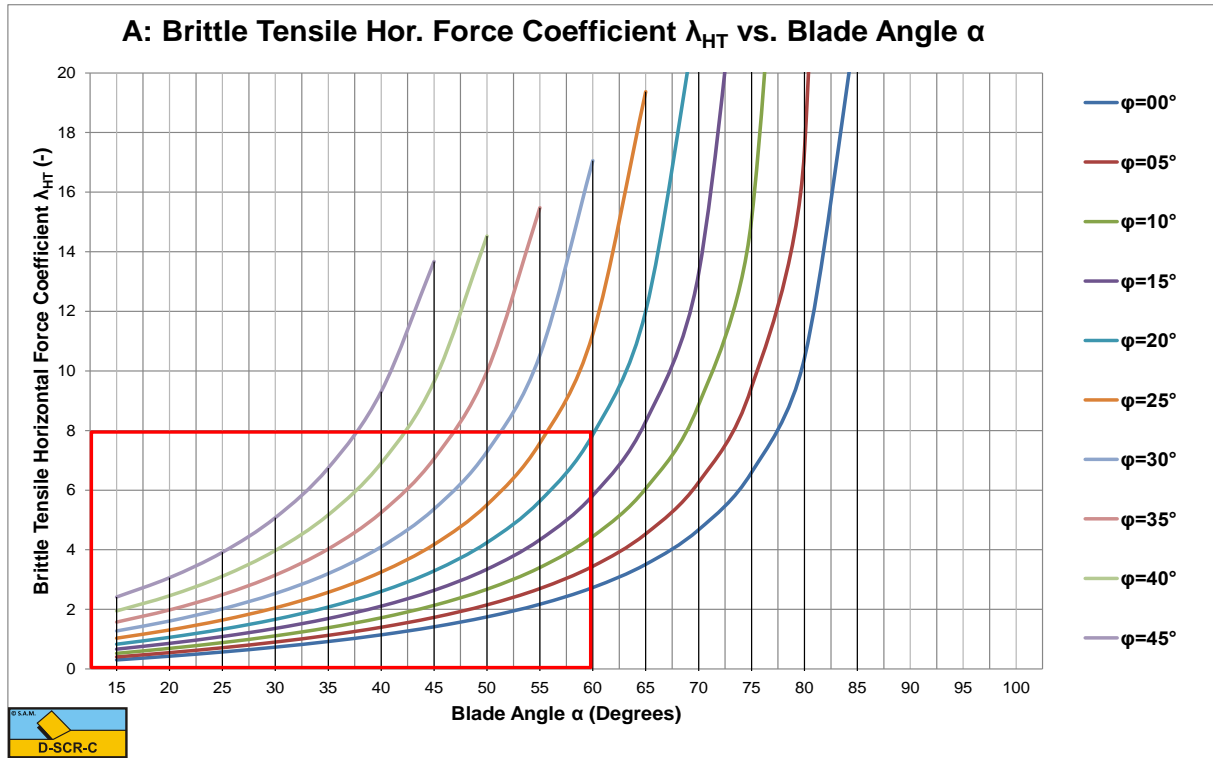
Figure W-31: The brittle (tensile failure) horizontal force coefficient \lambda_{HT} .
