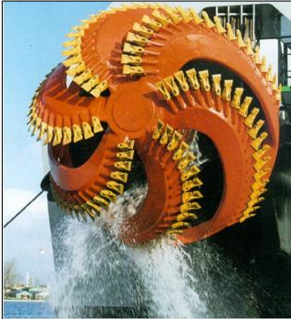
Figure Y-12: A sand cutter head.
