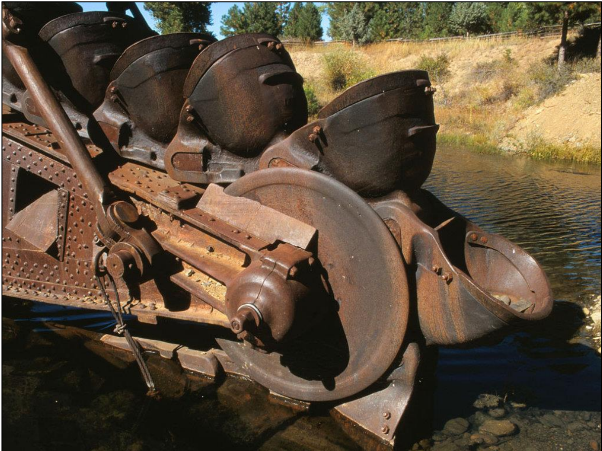
Figure Y-7: The buckets of a gold dredge.
