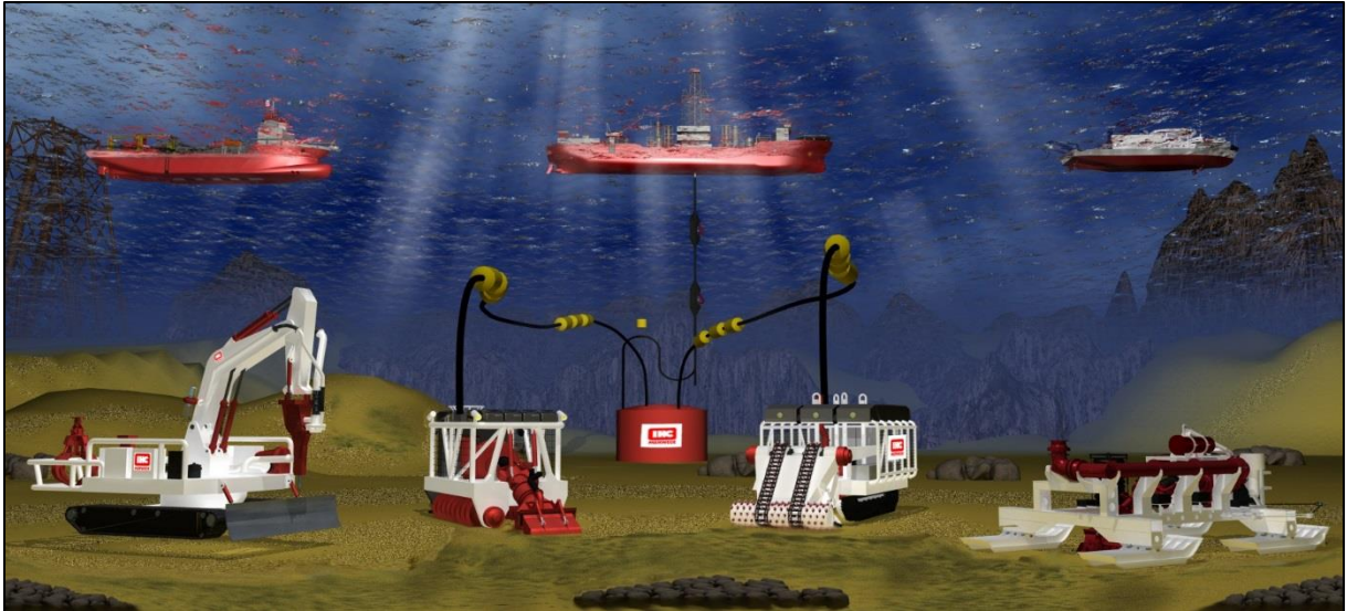
Figure Y-47: Deep sea mining excavators (IHC).
