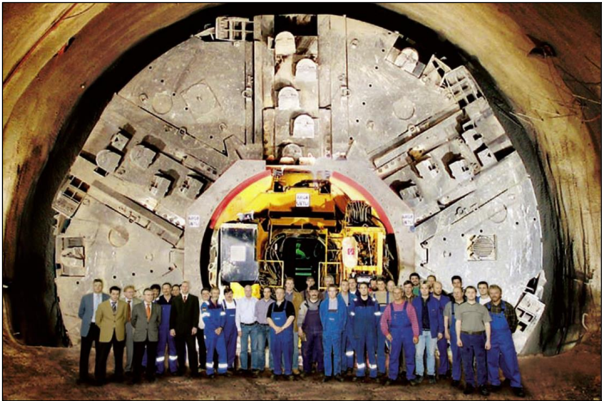
Figure Y-76: An integrated TBM.
