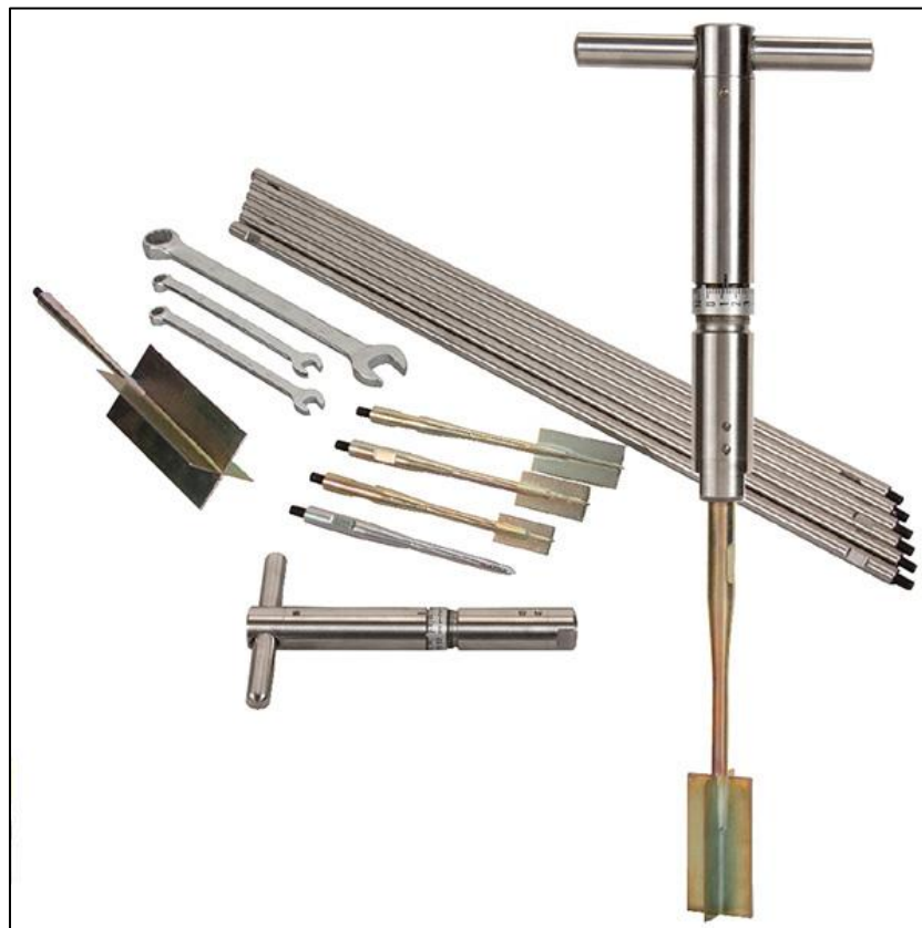
Figure 2-39: Shear vane and Torvane for soil testing (www.humboldtmg.com).
