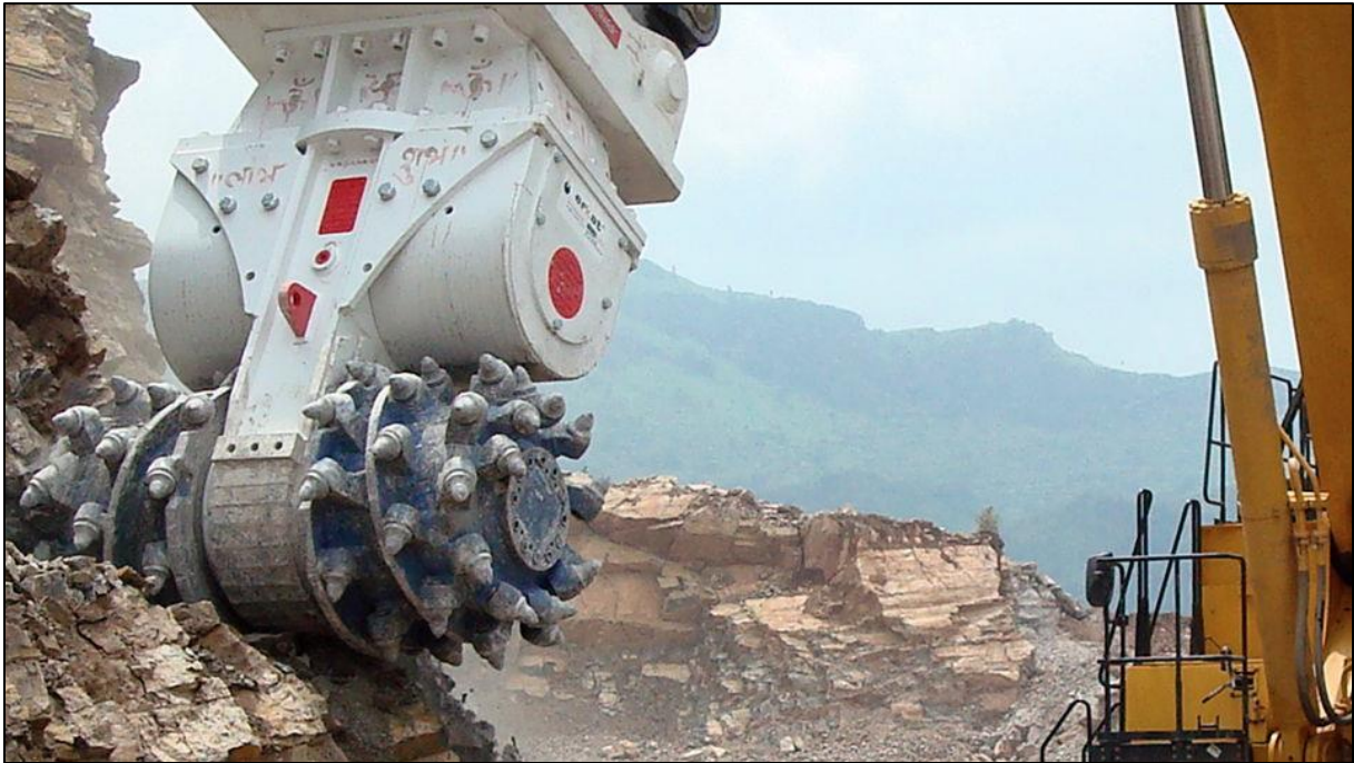
Figure Y-72: Double head drum cutter ( www.drumcutters.com ).
