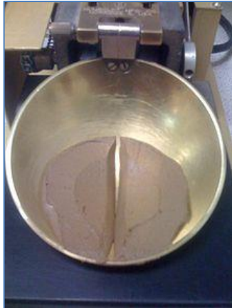
Figure 2-19: Liquid limit device.
