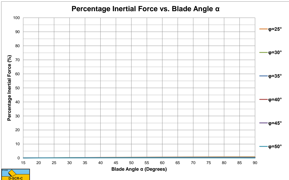
Figure 5-13: The percentage inertial force for a layer thickness h_i=1.0 m, blade height h_b=1.0 m and a cutting velocity v_c=0.5 m/sec.
