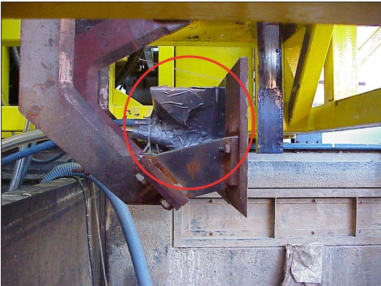
Figure 12-33: Cover with camera behind the blade.
