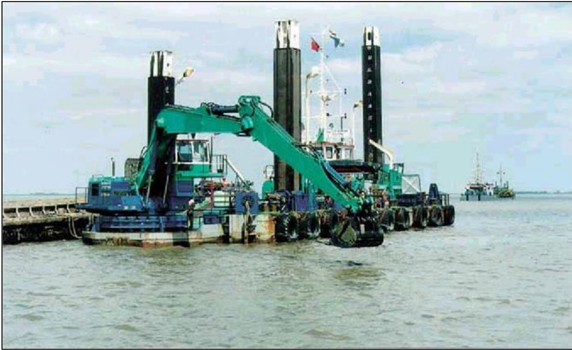
Figure Y-26: A large backhoe dredge.
