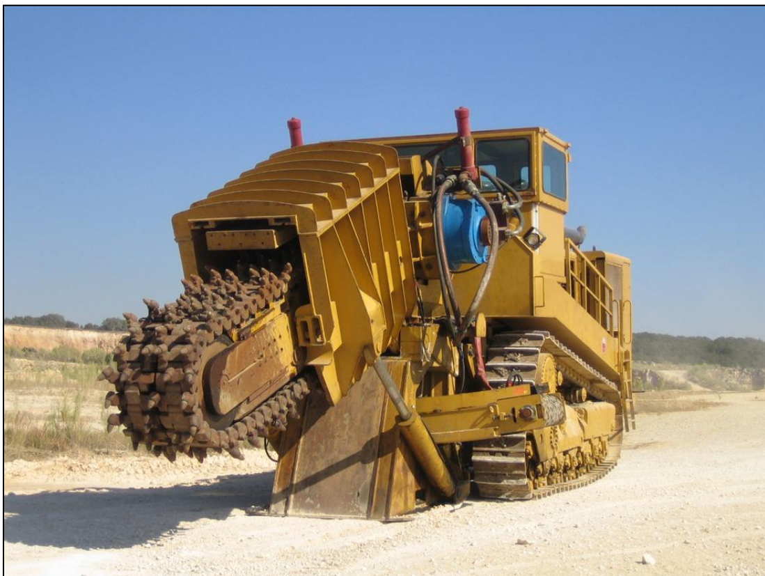
Figure Y-61: Rock trencher (Rocksaw International).
