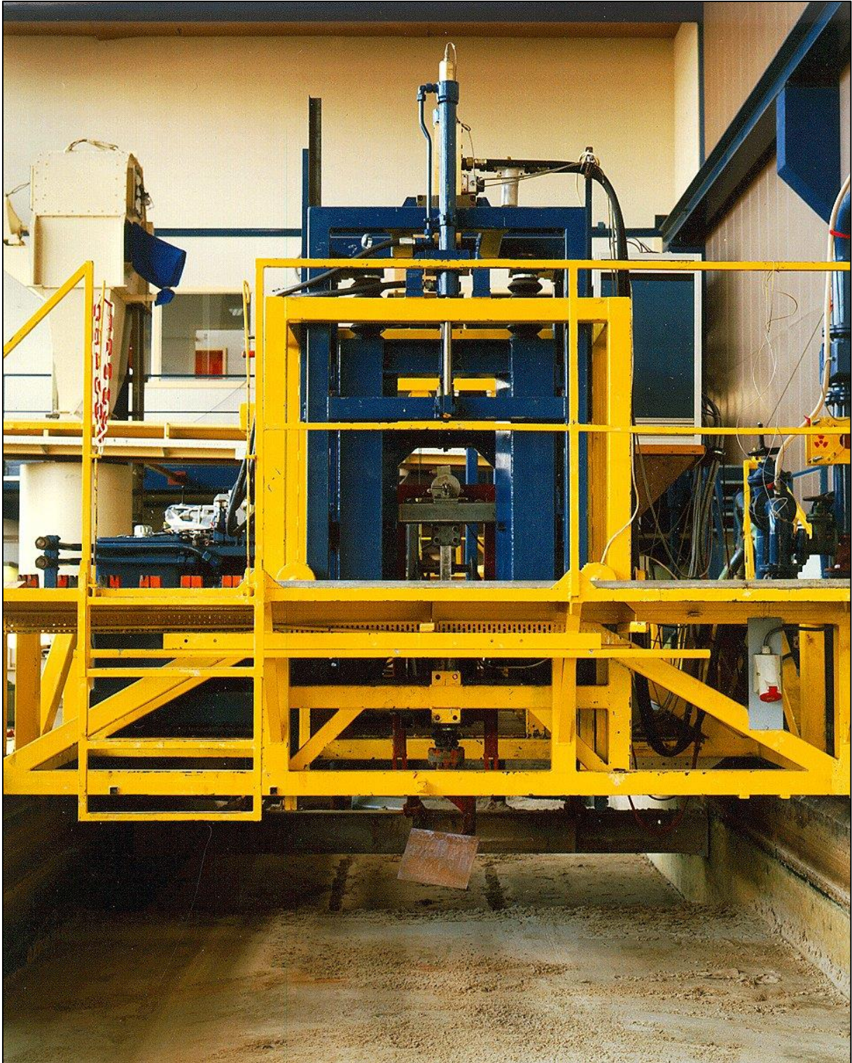
Figure 6-44: A blade mounted under the carriage in the new laboratory DE.
