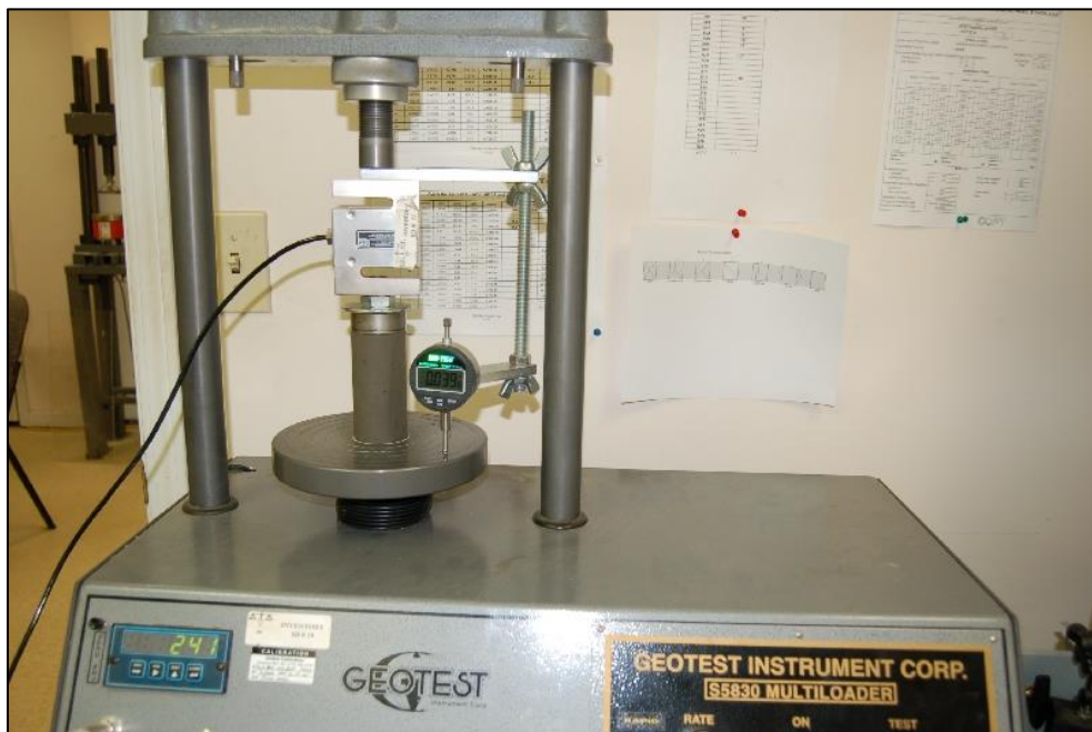
Figure 2-24: A UCS test facility (Timely Engineering Soil Tests, LLC).
