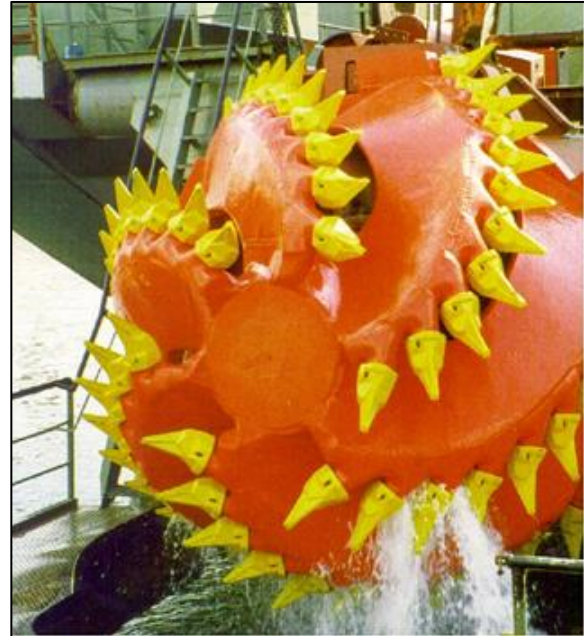
Figure Y-13: A rock cutter head.
