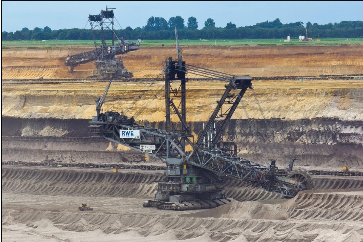
Figure 5-18: A dredging wheel used in the German braunkohl mines ( www.wikiwand.com ).
