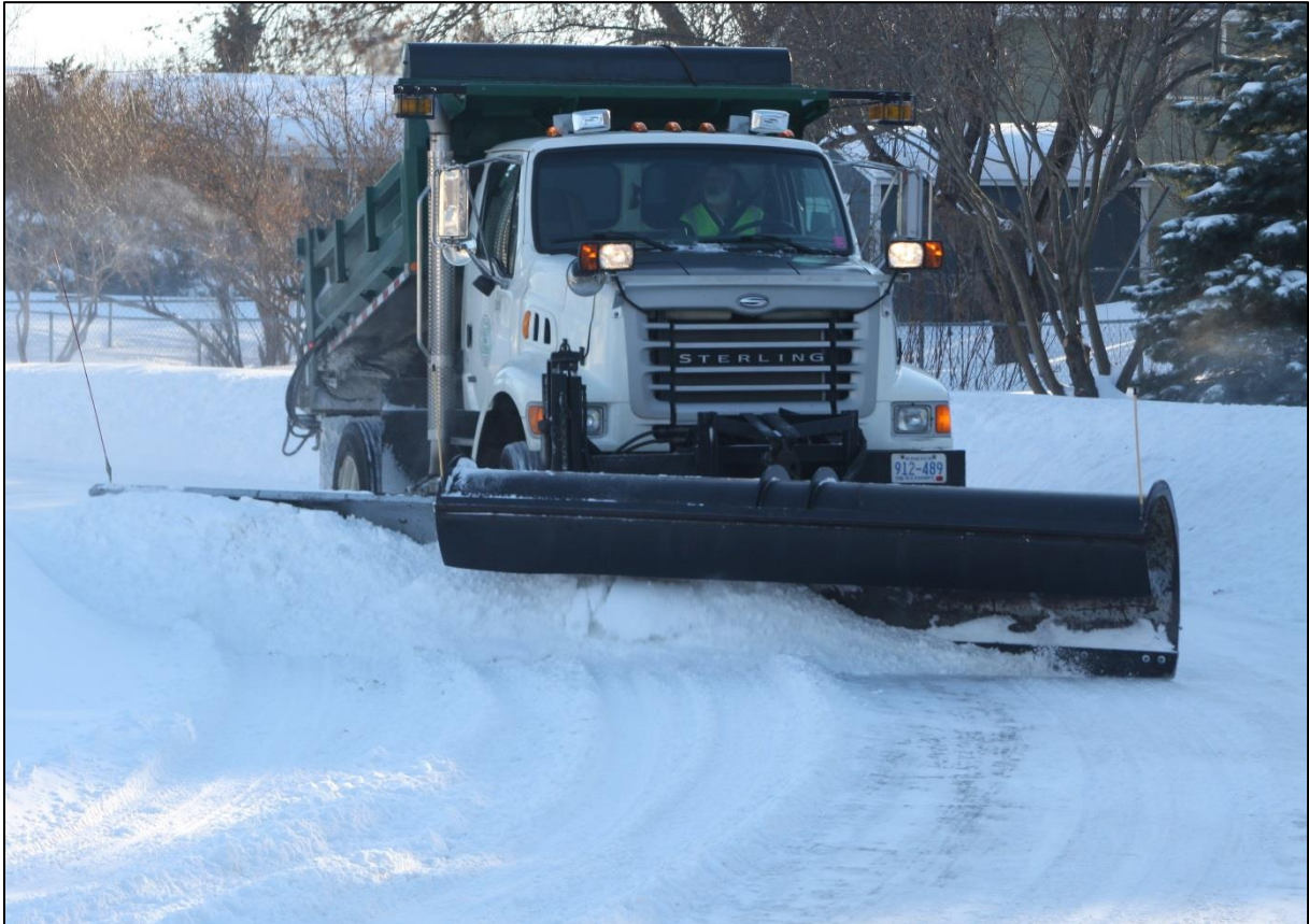
Figure 3-15: Urban winter service vehicle with snowplow (commons.wikimedia.org).
