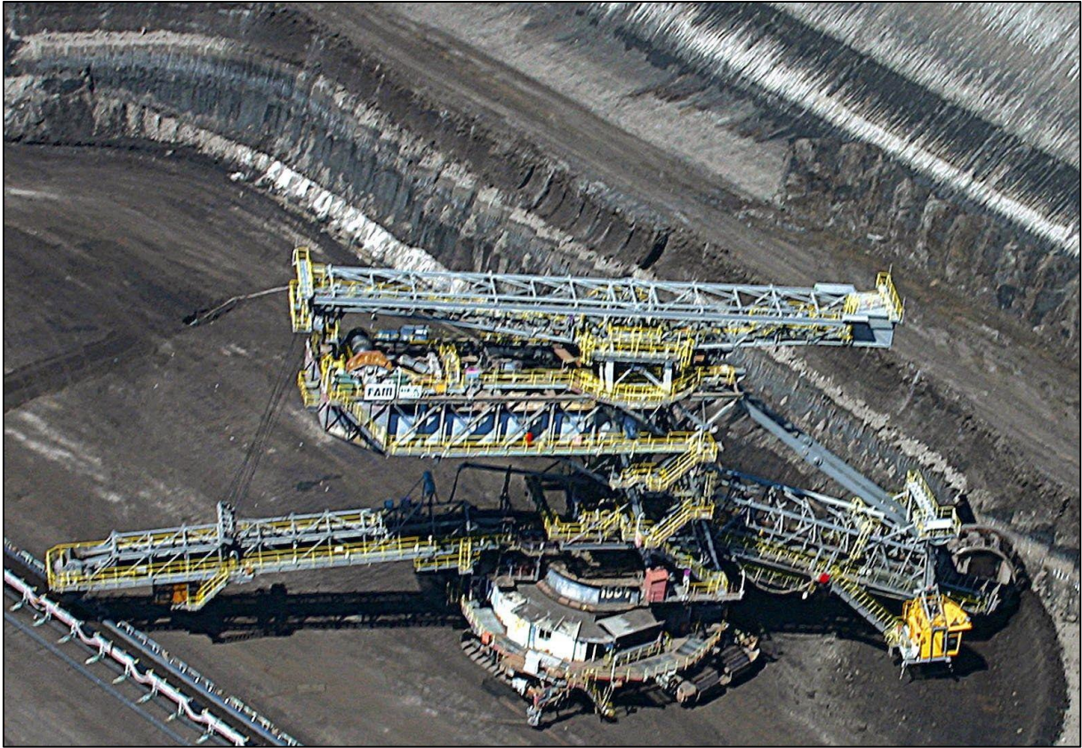
Figure Y-43: A bucket wheel excavator ( www.directindustry.com ).
