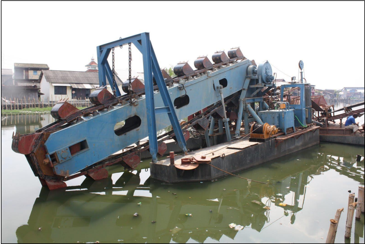
Figure Y-6: Garbage bucket dredge (Hamson Indonesia).
