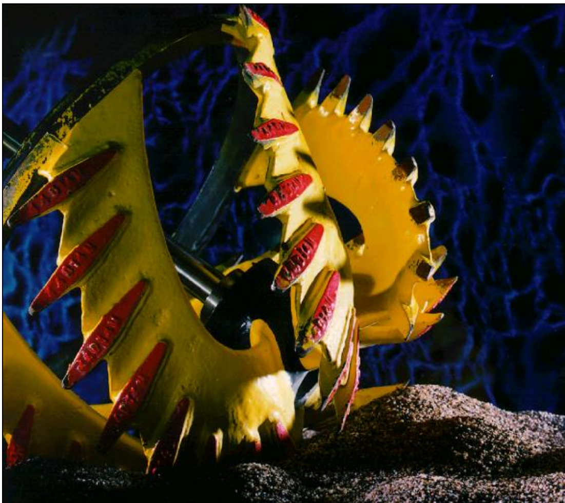
Figure Y-11: A model rock cutter head (Delft University of Technology).
