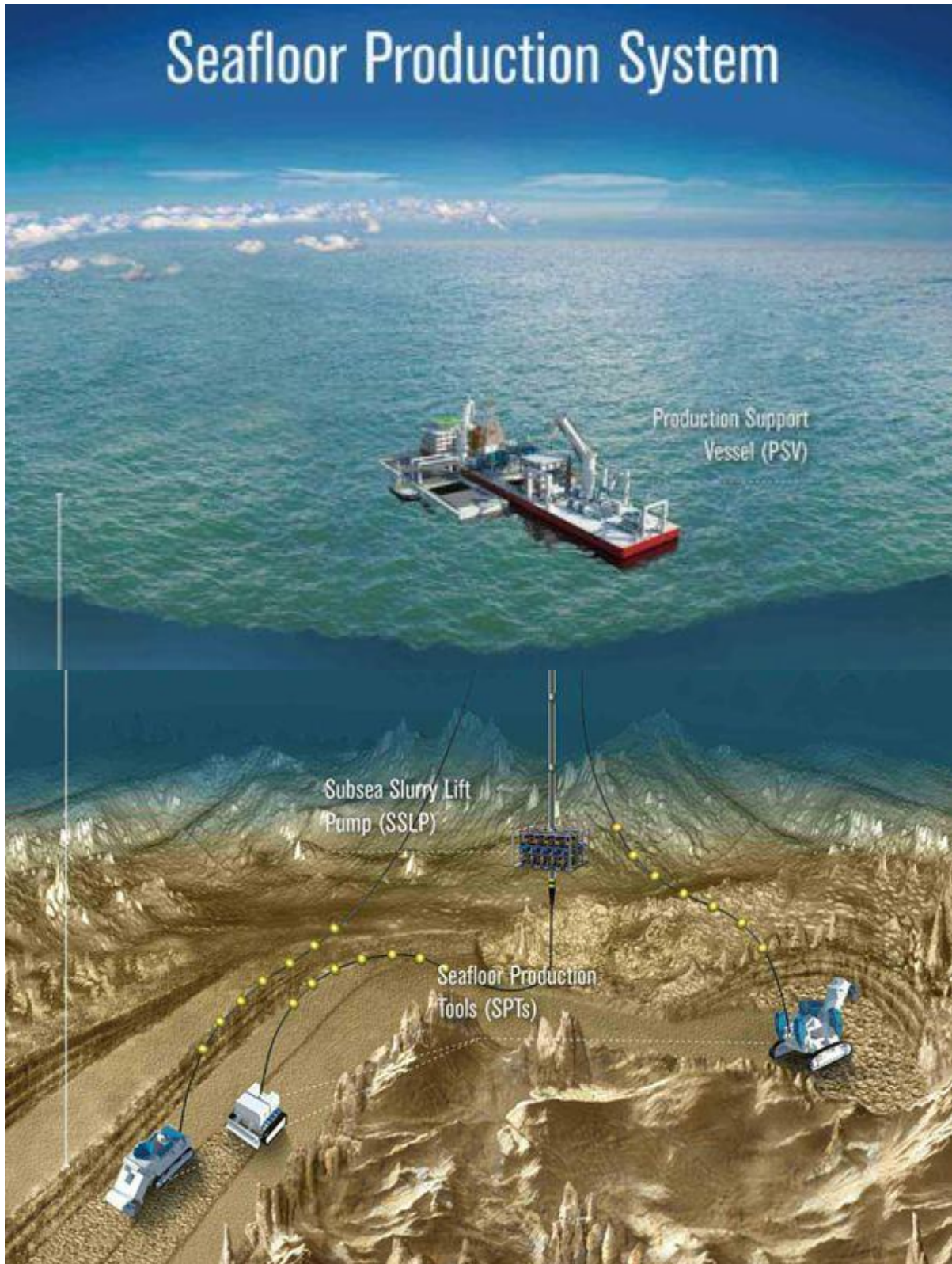
Figure Y-49: Sea floor production system.
