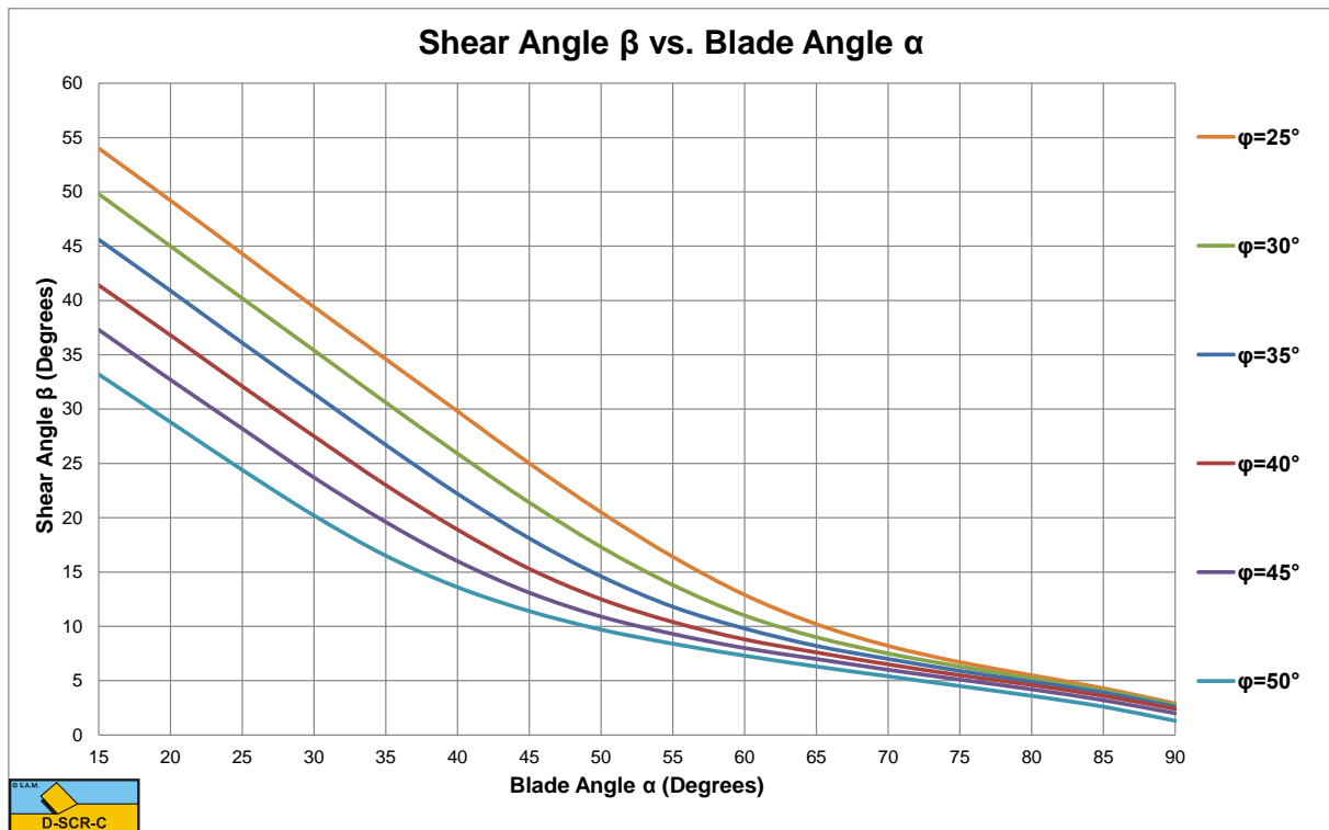
Figure B-24: The shear angle \beta , including the effect of inertial forces for a dimensionless inertial effect parameter \lambda_i=250 .
