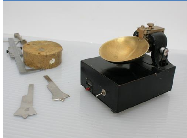
Figure 2-20: Liquid limit device.
