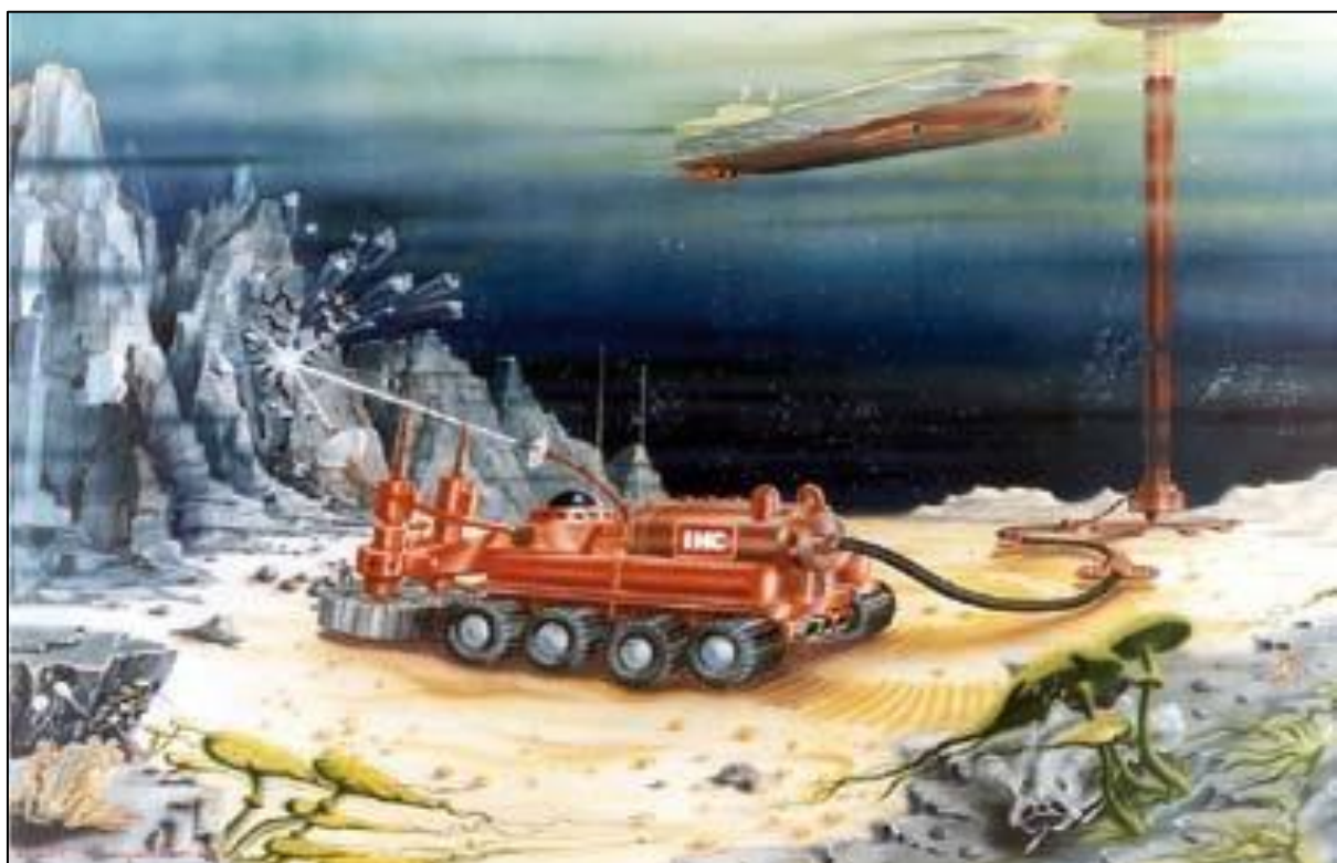
Figure Y-46: A deep sea mining excavator (IHC).
