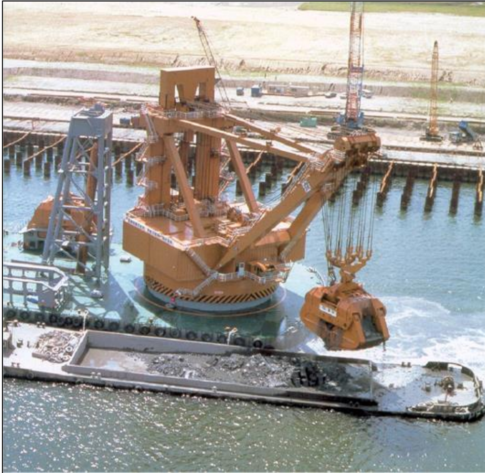
Figure Y-33: The biggest clamshell in the world.
