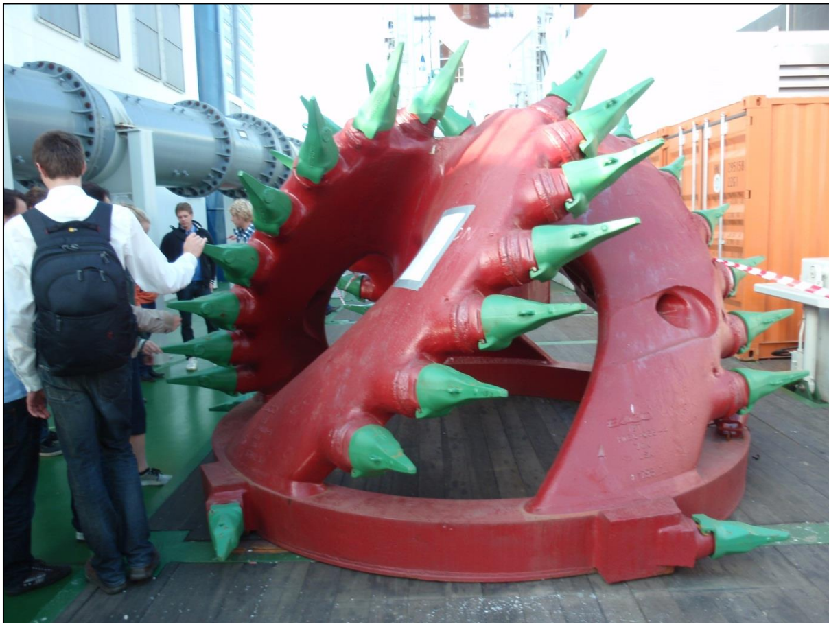
Figure Y-14: A rock cutter head (van Oord).
