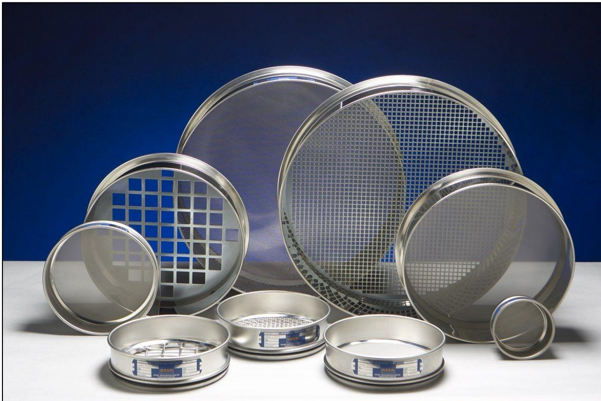
Figure 2-30: A set of sieves (Essa Australia from: www.directindustry.com ).
