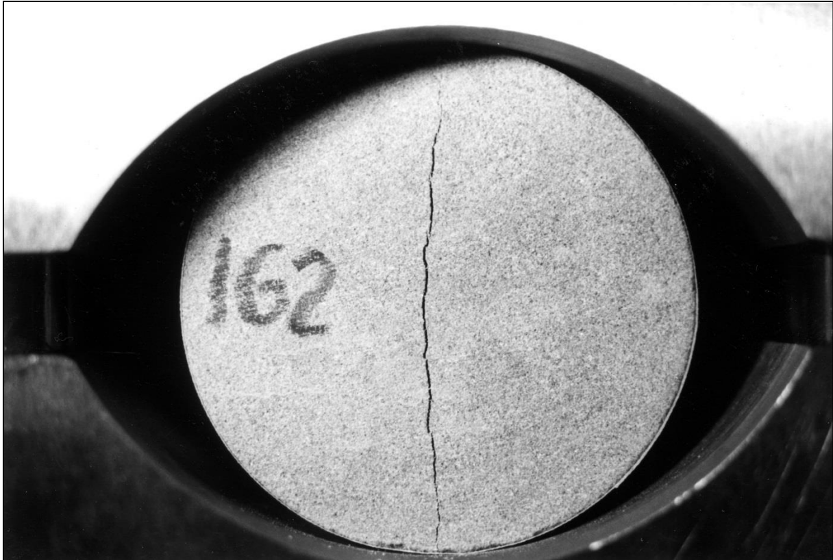
Figure 2-43: A BTS test after failure.
