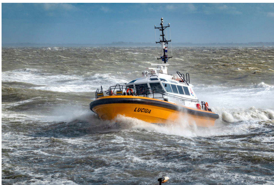
Figure 3.9: Wind-generated gravity waves at sea, probably Beaufort 5. Photo from Rijkswaterstaat ('Credits' on page 575).
