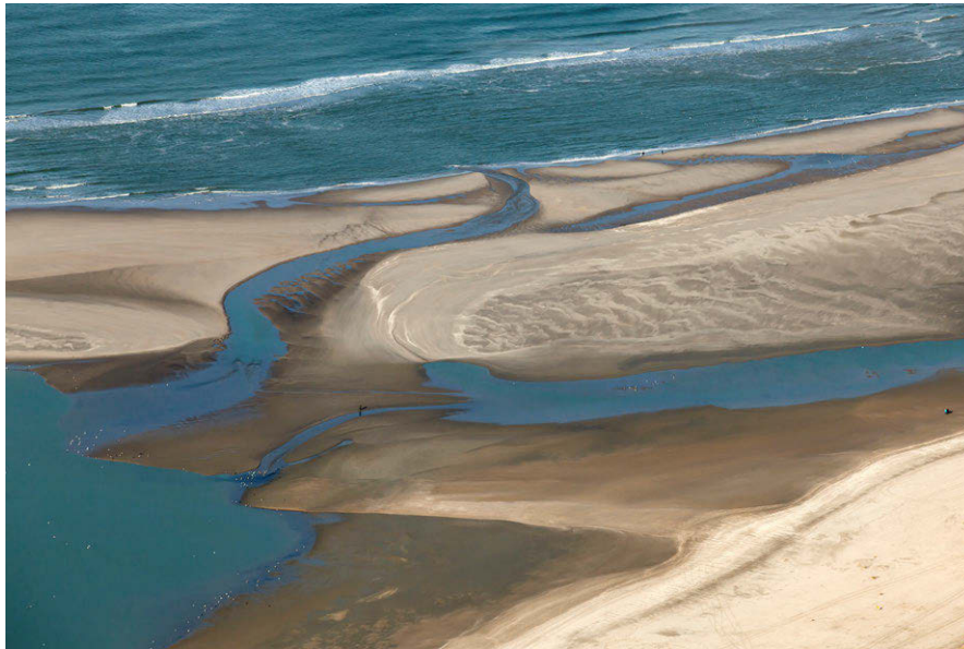
Figure 7.9: Ridge (intertidal bar) runnel (drainage channel) structure at low water at the northern flank of the Sand Engine on 16 February 2016. Photo by Jurriaan Brobbel, Rijkswaterstaat ( ‘Credits’ on page 575).
