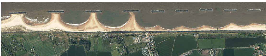
Figure 10.17: Series of emerged detached breakwaters in Sea Palling, England. Note the salients and tombolos. Vertical aerial photography obtained in May 2019. From UK Environmental Agency (‘Credits’ on page 575).
