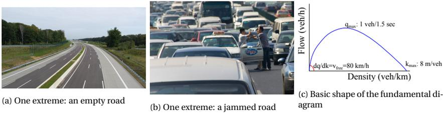
Figure 3.1: The extreme situations and an idea for the fundamental diagram
