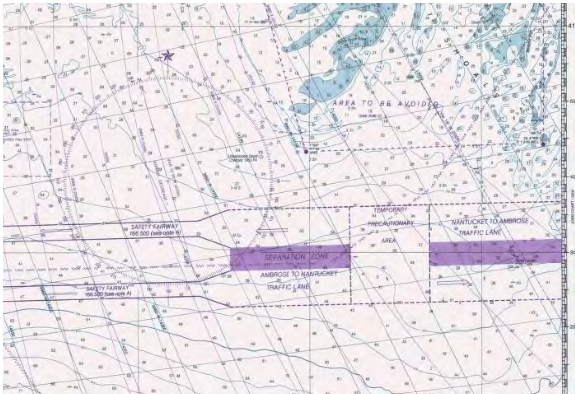
Figure 5.8: Example of a TSS ( Chart1 by Wikimedia commons is licenced under CC0 1.0).
