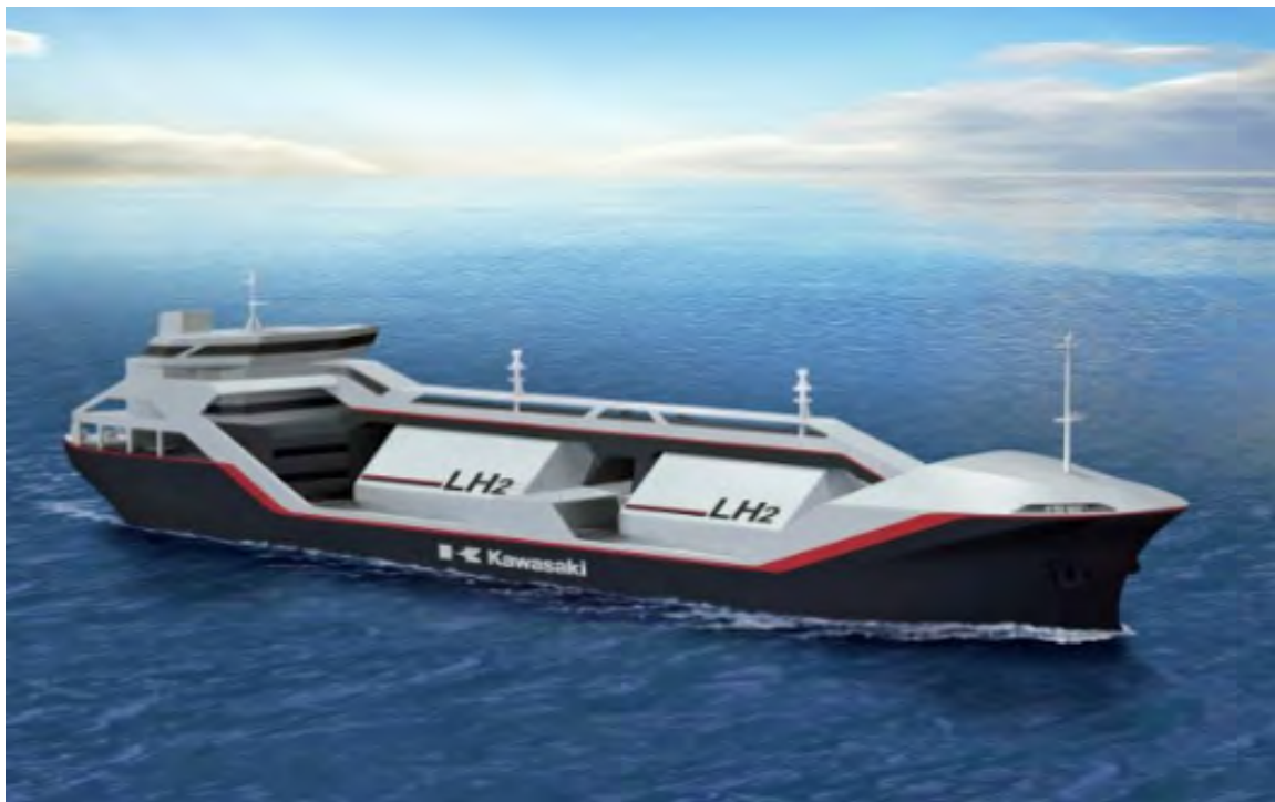
Figure 1.1: Artist impression of the world's first liquefied hydrogen carrier, the Suiso Frontier, (actually launched December 2019) (© Kawasaki Heavy Industries).
