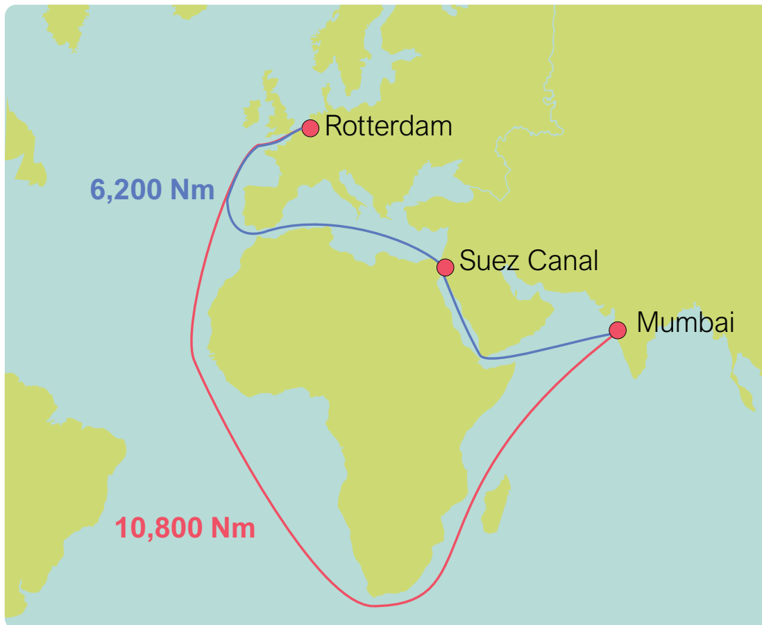
Figure 1.4: Route between Europe and Asia shortened by the Suez canal (by TU Delft – Ports and Waterways is licenced under CC BY-NC-SA 4.0).
