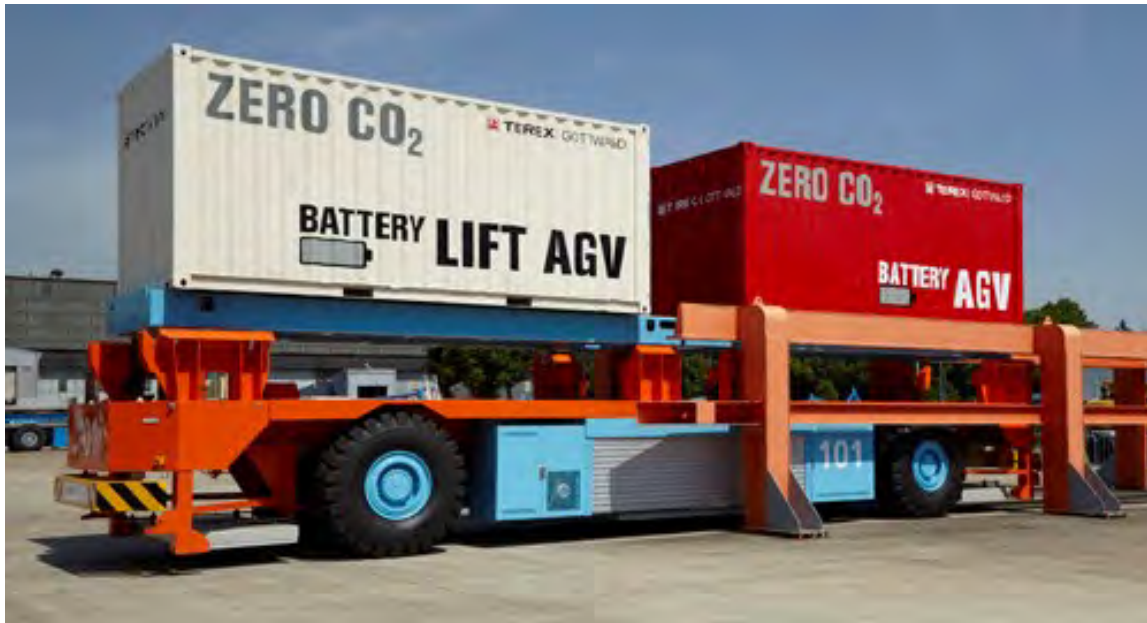
Figure 4.21: Lift Automated Guided Vehicle (Lift-AGV) (from www.konecranes.com , “Lift AGV”, Copyright by 2021 Konecranes).
