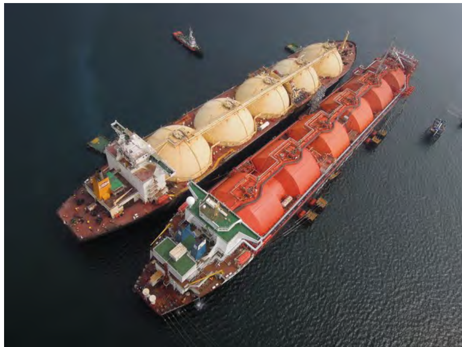
Figure 5.10: Offshore moored FSRU with an LNG-tanker alongside, West Java, Indonesia (Offshore LNG import terminal mooring in Indonesia by Royal HaskoningDHV is licenced under CC BY-NC-SA 4.0).
