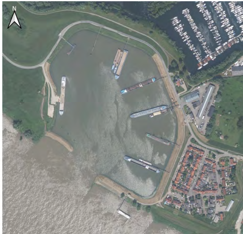
Figure 5.37: Lobith (NL), overnight harbour with floating landing stages (aerial imagery by the National Georegister (NGR) is licenced under CC BY 4.0).
