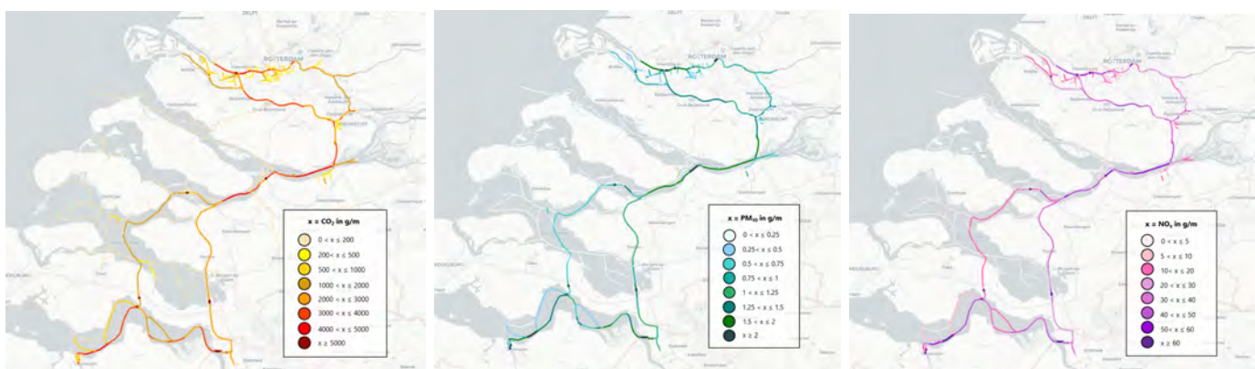
Figure 5.14: Potential \text{CO}_2 , \text{PM}_{10} and \text{NO}_x emissions, for September 2 nd , 2019, based on AIS data, projected on the transport network (images by Segers, 2021, are licenced under CC BY-NC-SA 4.0).
