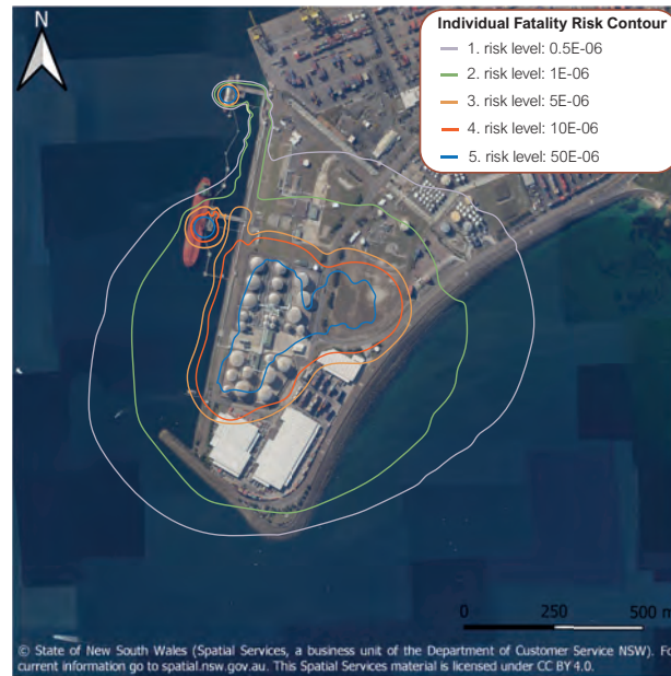
Figure 2.18: Individual fatality risk contours for an oil terminal, Port Botany, Australia (background: Spatial Service State of New South Wales, contours: Sherpa consulting, image by TU Delft – Ports and Waterways is licenced under CC BY-NC-SA 4.0).
