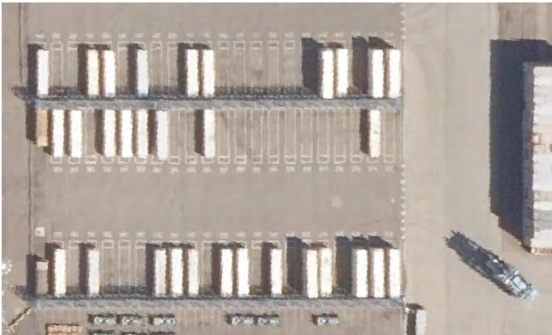
Figure 4.35: Example: reefers stack operated by straddle carriers (aerial imagery by the National Georegister (NGR) is licenced under CC BY 4.0).
