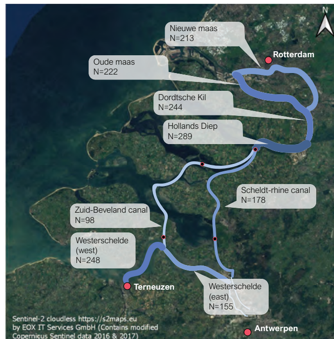
Figure 5.12: Traffic intensity as derived from AIS for the Rotterdam-Antwerp corridor for September 2 nd , 2019 (image modified from Segers, 2021, by TU Delft – Ports and Waterways is licenced under CC BY-NC-SA 4.0).
