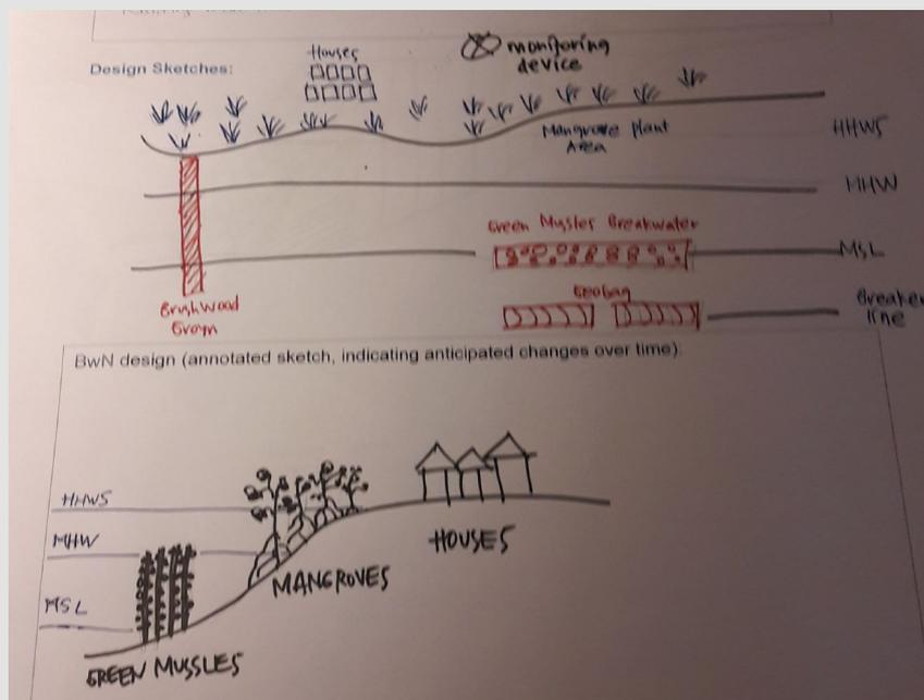
Design for a bamboo and green mussel breakwater located around mean sea level (MSL) with a geobag breakwater offshore of this and a mangrove planting area inshore of the shelter provided by the geobags and green mussels.
