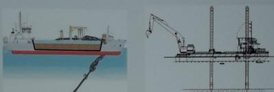
*Trailing suction hopper dredger and backhoe dredger.*
