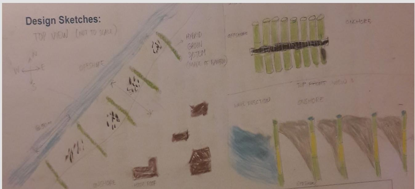
Design for cross-shore permeable groynes to be extended as sediment accretes nearer the coast. Photographs of the maquettes made to represent the design are included next.
