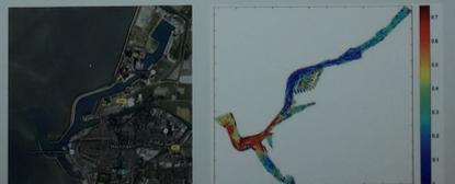
*The harbour of Harlingen and an overview of the measured silt layer thickness.*
