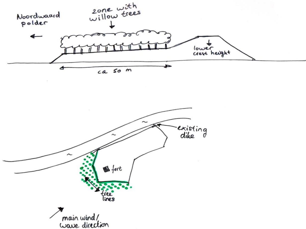
Using a 50 m zone of willow trees will lead to an approximately 70% reduce of wave height = 0,84 meter instead of 1,2 m. This means the total crest height will be reduced by ca. 20 cm (which I think is not really a lot actually).
