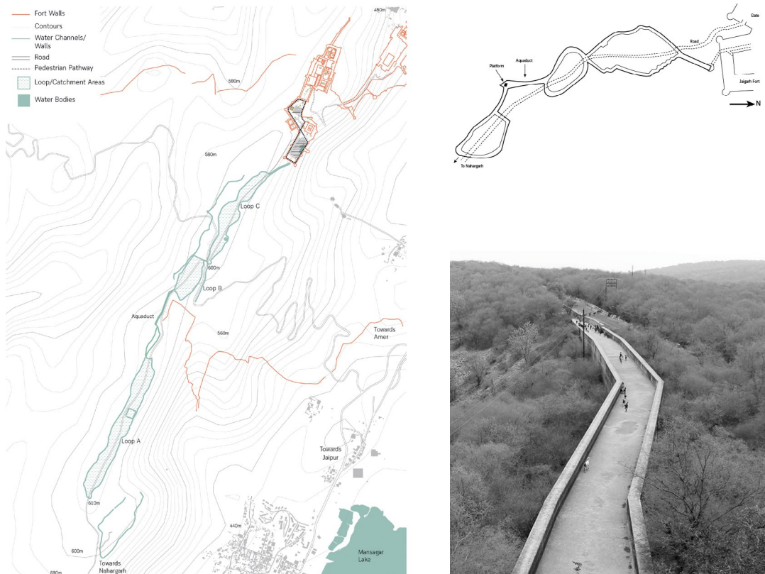
Fig. 14 Detailed catchment network of the Jaigarh water system (plan), conceptual diagram of the system, and a photograph of the water channel entering the fort. Adapted from Chandna (2019).
