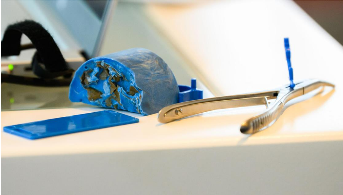
Figure 1. Closed Loop Recycling: GO Jack Instrument Opener made from recycled blue wrap hospital waste and reused as new product in the same hospital.
