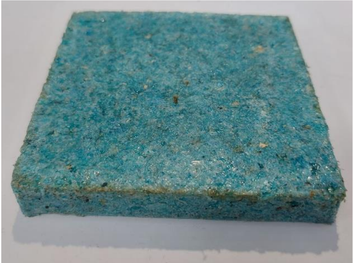
Figure 20: A standardized end product (tile) which can be used for further testing of material properties.
