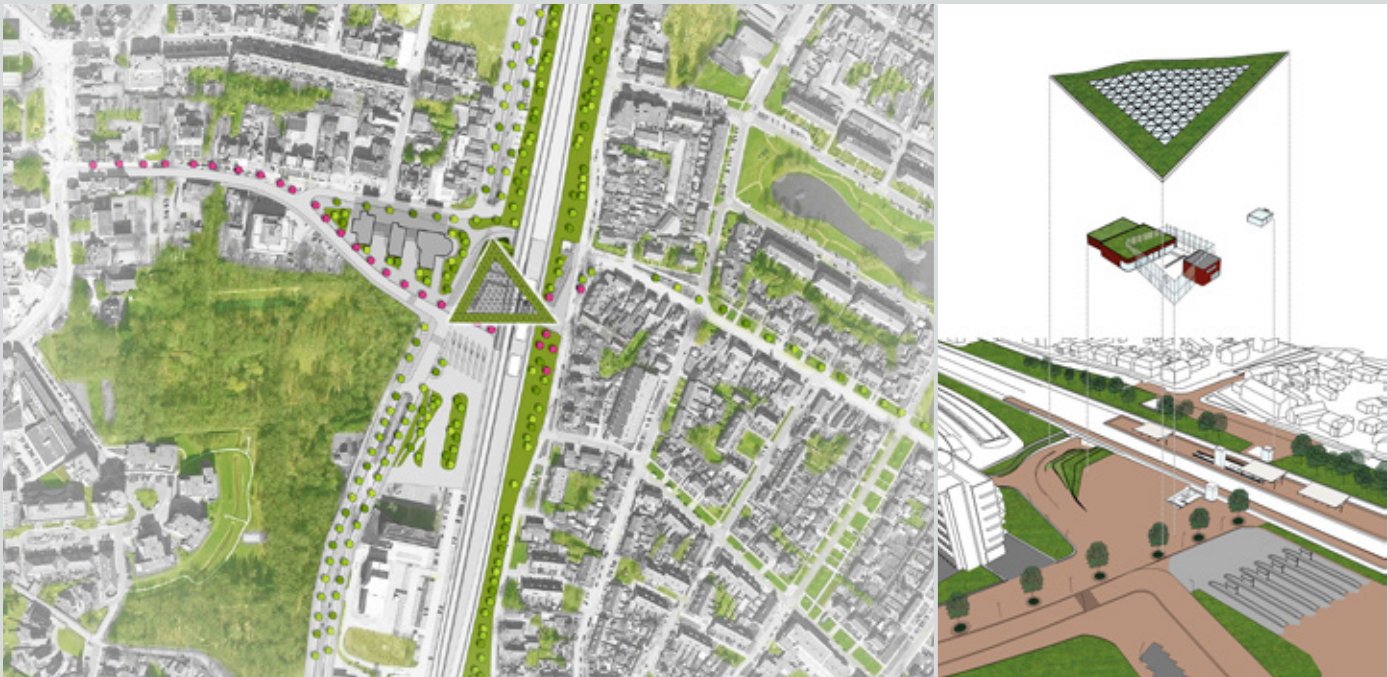
The station and square are part of the urban development FlorijnAs and are connected to the city center. Through car traffic goes through a tunnel under the station square / Cross-section with roof, platforms, facilities, pedestrian underpass, bicycle parking and access on two sides. [© De Zwarte Hond]
