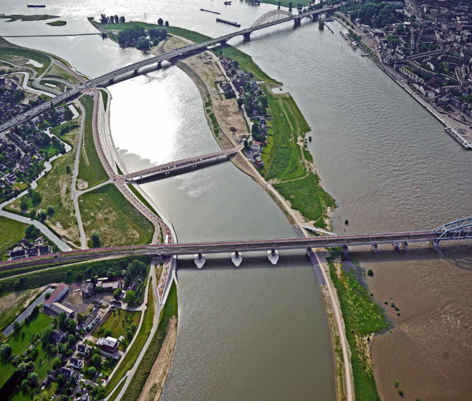
The bypass of the Waal River at Lent, Nijmegen, which aims to reduce the water level in winter and offers recreational use in summer at lower water levels. [© Rijkswaterstaat, Johan Roerink] / Excavation at the IJssel River for floodplains and nature near the city of Arnhem. [© Rijkswaterstaat, Room for the River] / Port of Tholen at the Volkerrak Zoommeer in Zeeland: water storage during the period when flood defences on the coast are closed and there is excess water from the rivers; also suitable for recreational use. [© Rijkswaterstaat, Room for the River]
