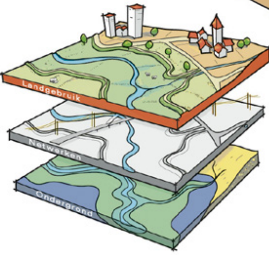
Three examples show the evolution of the layer model with layers like the layer approach, but from a different starting point and with a different use. The subsurface forms the first layer, the infrastructure networks the second layer and land use the third layer. Top: one of the first examples primarily to distinct the layers. It does not show the relations between the layers. [© Dauvelliér Planadvies] / Left: the relationships between the layers are expressed, including the water system. [© BoschSlabbers] / Right: the final model redefines the first layer as the natural system and adds the atmosphere. [© H+N+S] / Below: Panorama Gelderse Rivieren: the Waal River. [© West 8]
