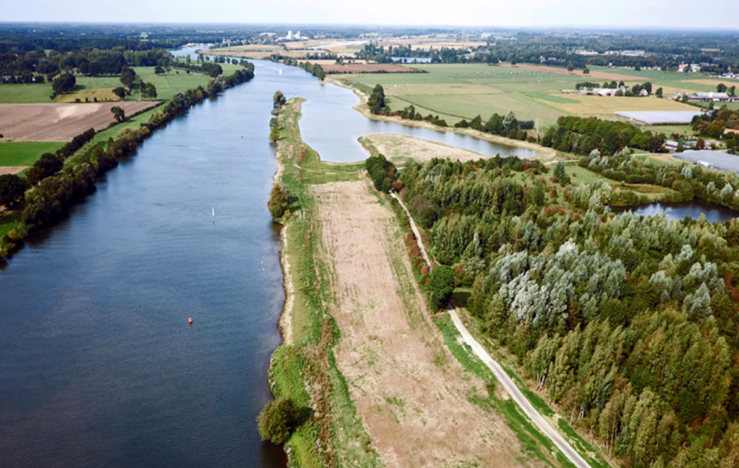
Figures 2–3. Well-Aijen Zuid, Limburg: high water discharge canal shown with the regular water level. [© Rijkswaterstaat, Joop van Houdt] / Discharge of high water via the discharge canal, February 2020. [© Rijkswaterstaat, Studio Retouched]
