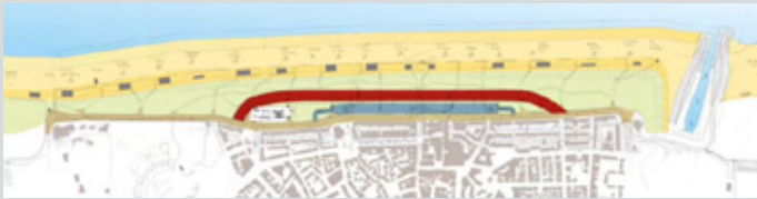
Left: Province of South Holland. [© Jan Willem van Aalst] / Right: map of the coastal zone at Katwijk aan Zee (NW direction on the top). The thick red line represents the dike in dune structure. The thick blue line enclosed by the dike and boulevard is the underground car park. / Below: top-view drawing of the coastal zone. The structures are embedded in the dune landscape. [© OKRA Landscape Architects]
