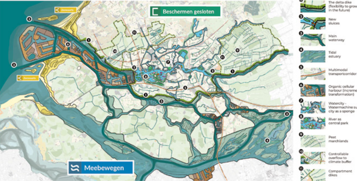
Rotterdam in 2200: vision by De Urbanisten et al. (2022) for the port and city in case of a sea level rise between 1 and 3 metres in 2100. The port will be fully accessible, but the city – as a Sponge City – will be closed off from the Nieuwe Maas River by sluices and delta dikes. The vision, as one of the cases in the Redesigning Deltas design study, incorporates the 'move along' and 'full closure' adaptation strategies to sea level rise as defined by Deltares. [© De Urbanisten]
