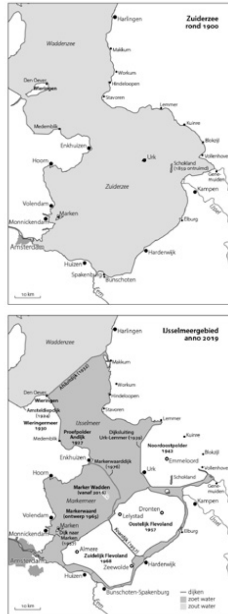
Figure 1. Design of the closure of the Zuiderzee and its phased reclamation by Cornelis Lely, 1892. [PD Zuiderzee collection] / Figure 2. The Zuiderzee around 1900 before the construction of the Afsluitdijk (top) and the IJsselmeer area around 2019, after its construction with the Wieringermeerpolder, Noordoostpolder and Flevoland (below). [© Margot Stoete]
