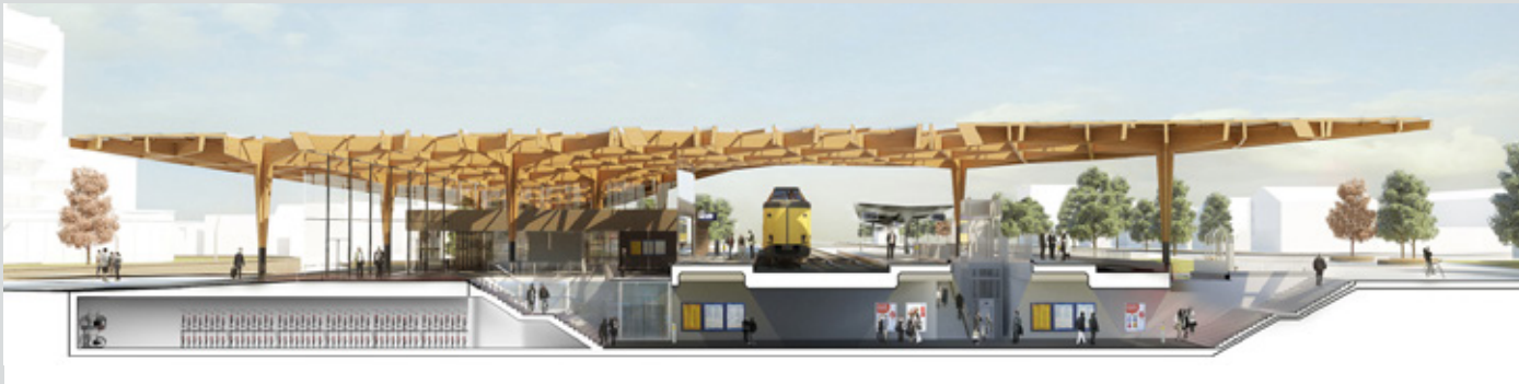
The station and square are part of the urban development FlorijnAs and are connected to the city center. Through car traffic goes through a tunnel under the station square / Cross-section with roof, platforms, facilities, pedestrian underpass, bicycle parking and access on two sides. [© De Zwarte Hond]
