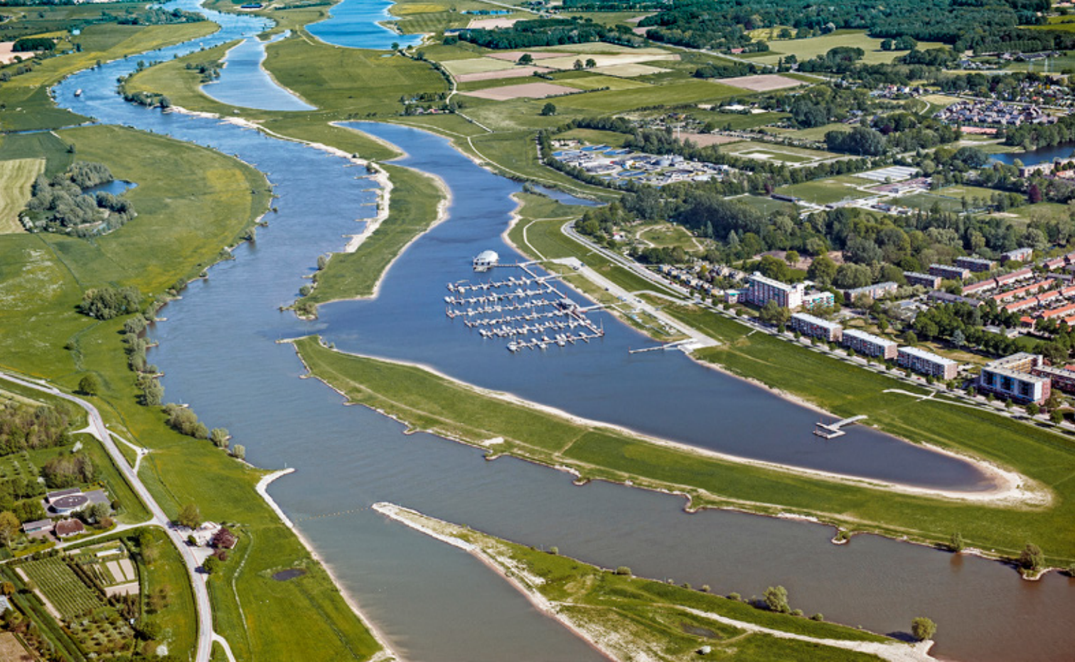
Deventer, Overijssel: new secondary canal in the floodplains of the IJssel River for extra discharge capacity combined with a marina. / North Holland: 3D printed concrete bicycle bridge for the reconstructed N243 road Alkmaar – Avenhorn. [© Witteveen+Bos]
