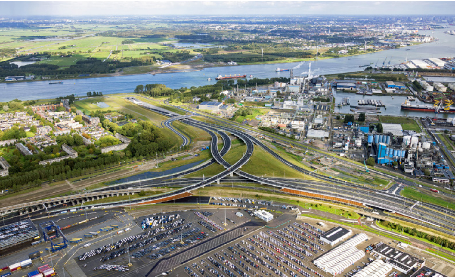
Blankenburgverbinding (A24): the Holland tunnel under the Zuidbuurt area, the viaduct of the Hoekse Lijn, and the sunken road along Krabbeplass towards the A20 on the north bank of the Nieuwe Waterweg (top). Connection of the A15 with the A24 and the Maasdelta tunnel between Rozenburg and the port on the south bank (bottom). [© Rijkswaterstaat, Topview Luchtfotografie]
