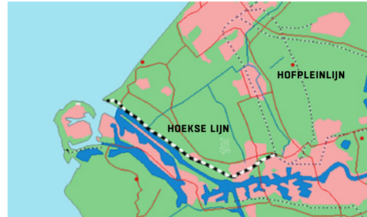
Figure 2. The Hofpleinlijn was the first railway line that was converted to a metro line, between Rotterdam and The Hague. The Hoekse Lijn has been converted between Schiedam and Hoek van Holland and integrated in the metro network of Rotterdam (black/white line).
