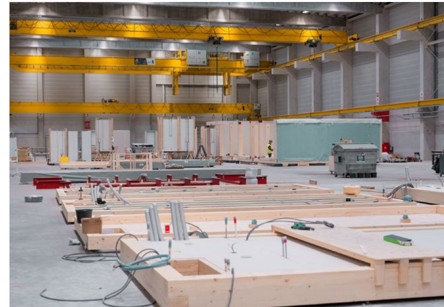
Figure 7 Modular mass timber housing factory (20,000 m 2 ) in the Netherlands, set to produce 1,500 houses a year (photograph by Lister Buildings).
