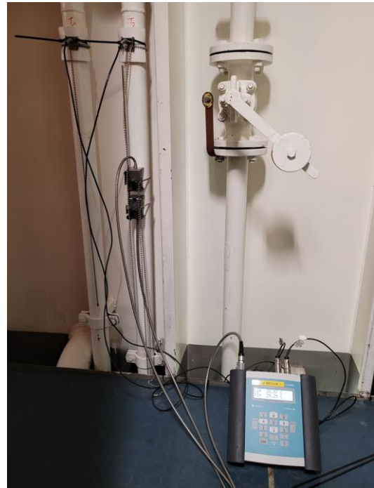
Figure 4: Setup of heat flow rate measurement from cooling of the battery's bidirectional converter
